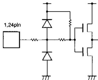
Input with pulldown resistors
