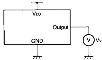
Fig. 5 Video signal output voltage measurement circuit
