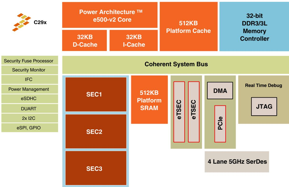
**Figure 3. C29x logical block diagram**
