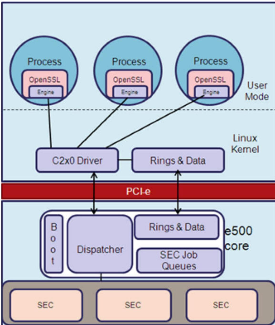
Figure 5. C29x PK Calculator software model
