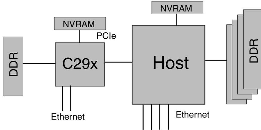
**Figure 2. C29x operating as secure key management module**
