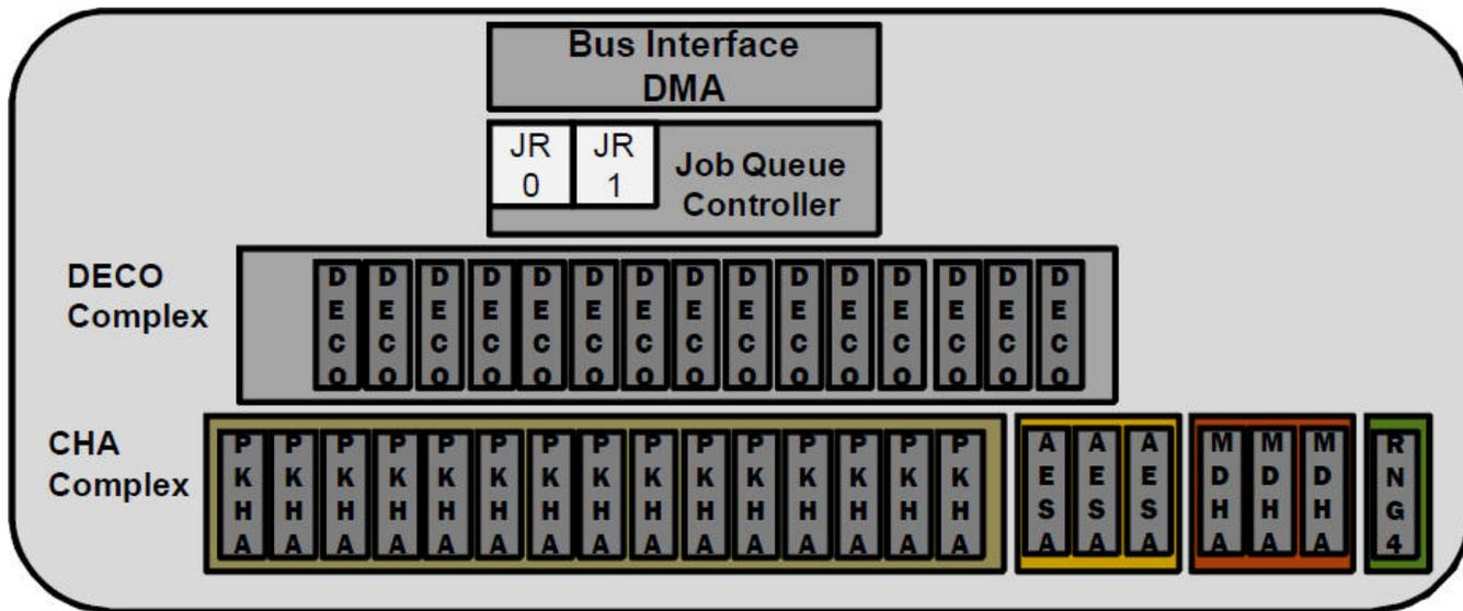
**Figure 4. SEC logical block diagram**
