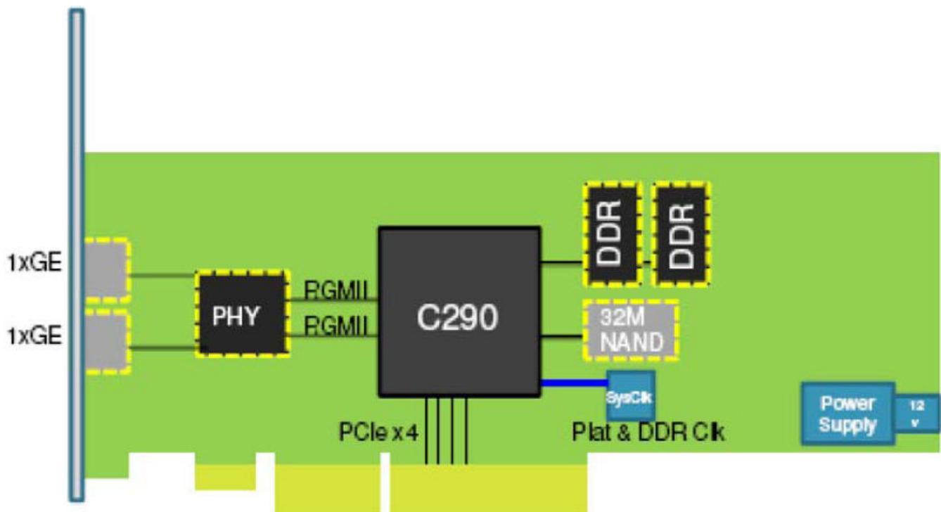
Figure 7. C29x half height PCIe card development system
