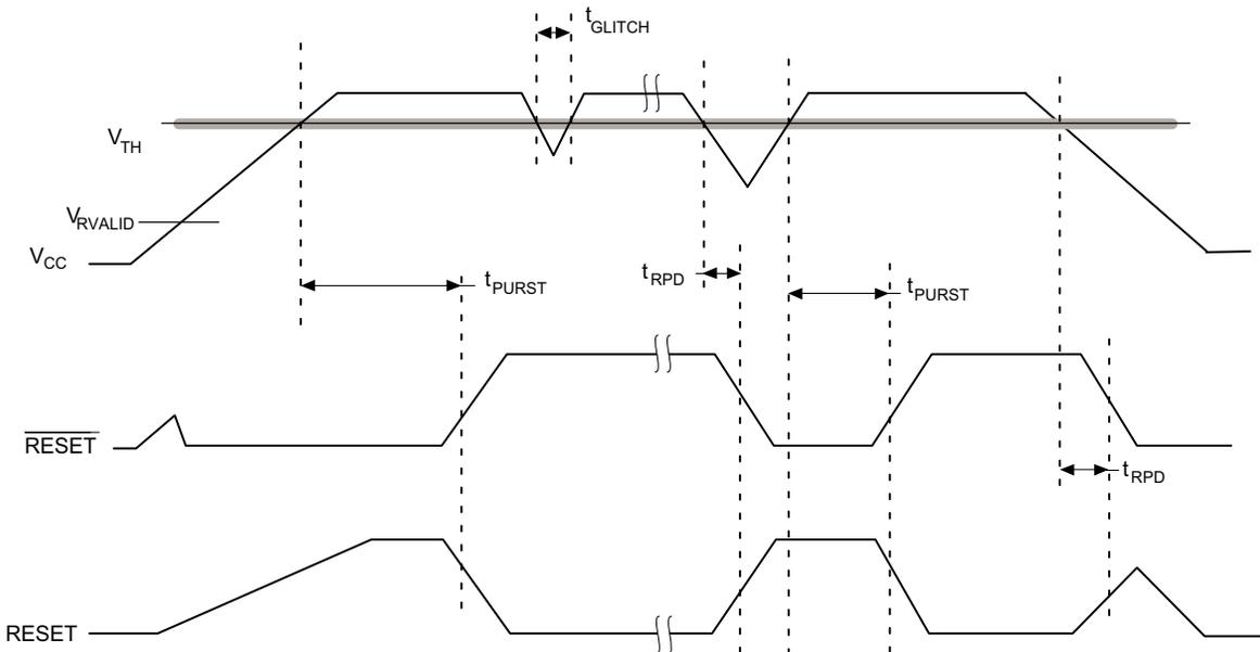
**Figure 1. RESET Output Timing**
