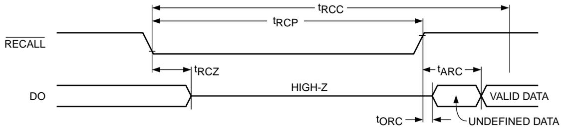
**Figure 6. Hardware Store Cycle Timing**
