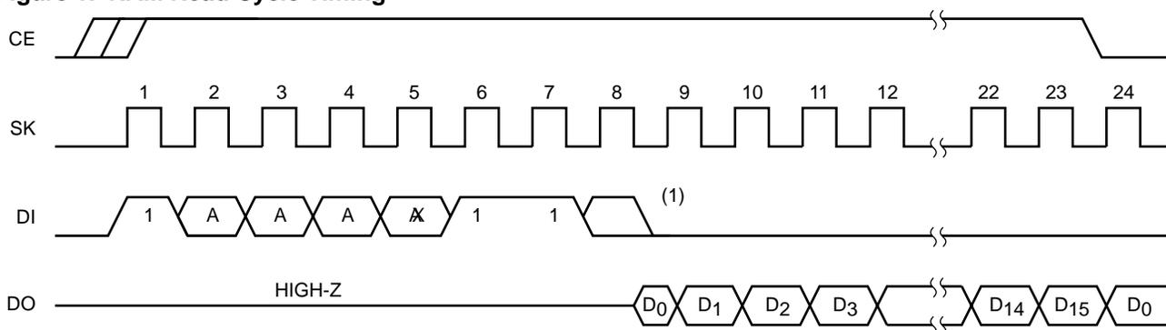
Figure 2. RAM Write Cycle Timing
