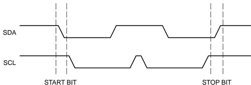
Figure 3. Start/Stop Timing
