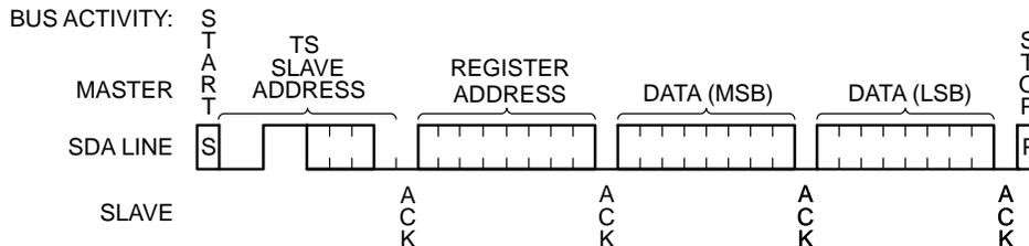
Figure 6. Temperature Sensor Register Write
