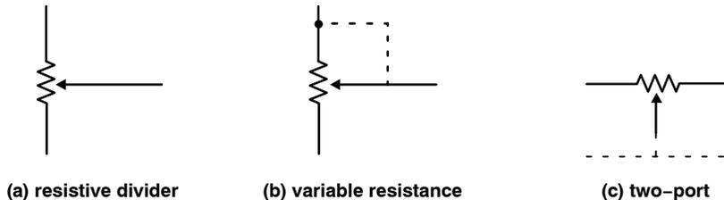
Figure 6. Potentiometer Configuration
