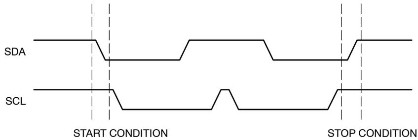
**Figure 4. Start/Stop Timing**
