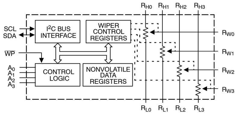
**Figure 1. Functional Diagram**
