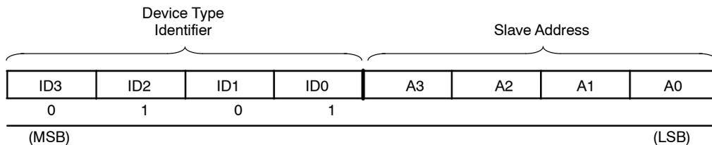
Figure 8. Identification Byte Format
