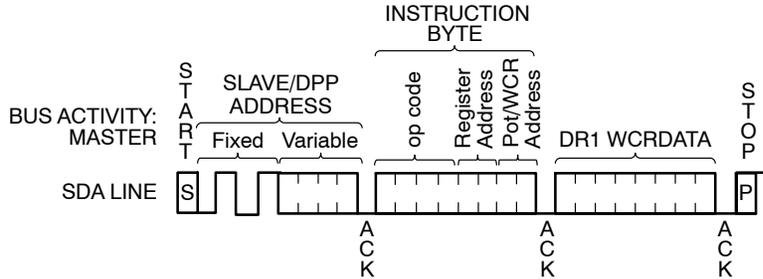
Figure 7. Write Timing
