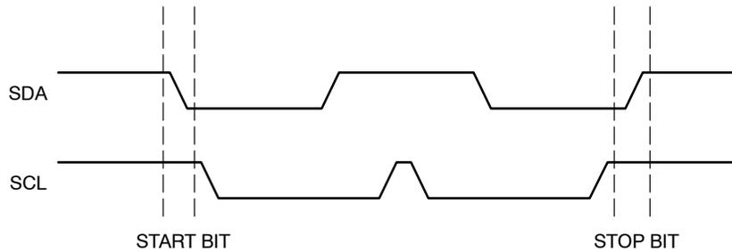
**Figure 4. Start/Stop Timing**
