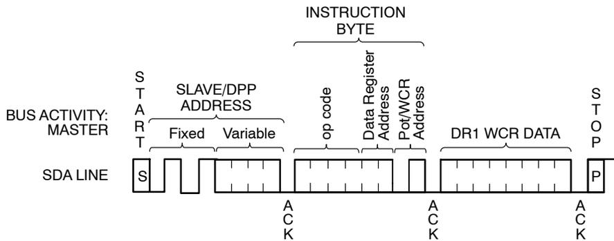
Figure 7. Write Timing
