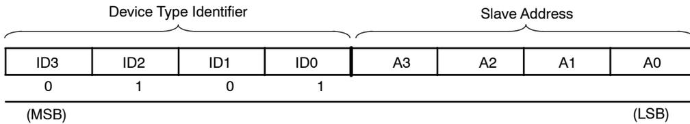
**Figure 8. Identification Byte Format**
