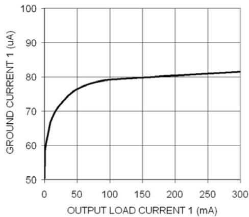
Figure 7. Ground Current (EN2 = GND)
