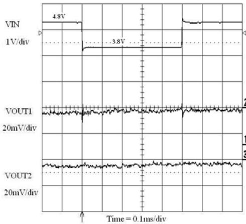
**Figure 28. Line Transient Response (100/0.1 mA Loads)**
