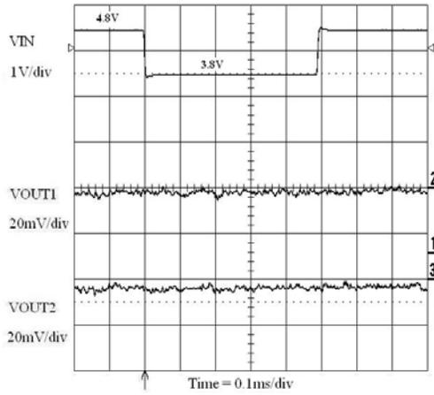
**Figure 26. Line Transient Response (0.1 mA Loads)**
