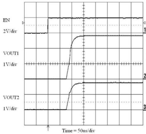
Figure 18. Enable Turn-on (100  $\mu\text{A}$  Loads)
