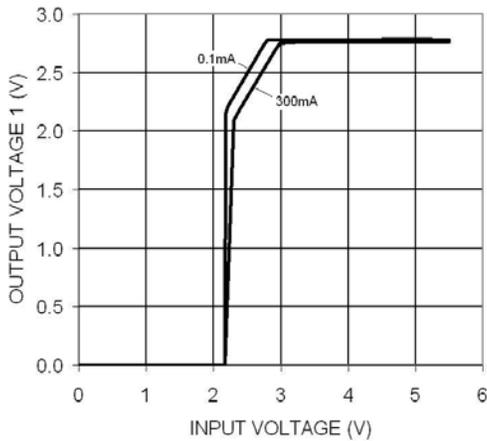
Figure 11. Output 1 Dropout Characteristics
