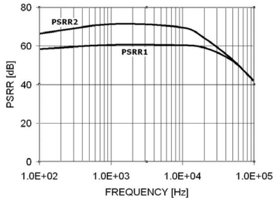
Figure 17. PSRR 1 & 2 vs. Frequency
