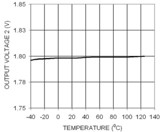
Figure 4. Output Voltage 2 vs. Temperature
