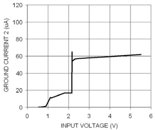
Figure 10. Ground Current (EN1 = GND)
