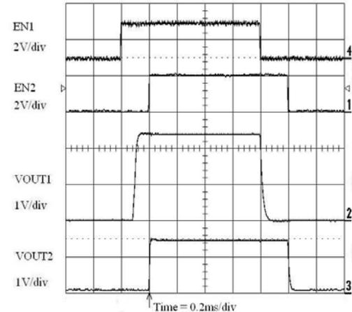
**Figure 29. Separate Enable Operation (100 mA Loads)**
