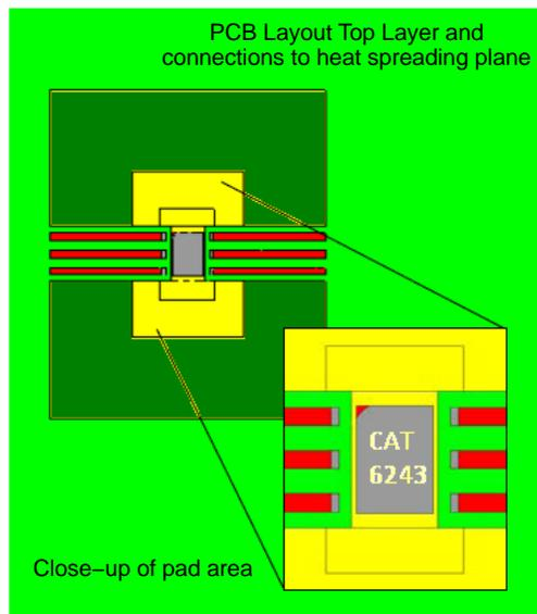
**Figure 29. Topside Copper Foil Pattern for Heat Dissipation**
