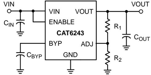
Figure 27. Adjustable Output Resistor Divider
