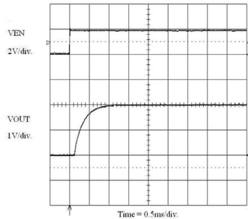
Figure 20. Enable Turn-On (1000 mA Load)
