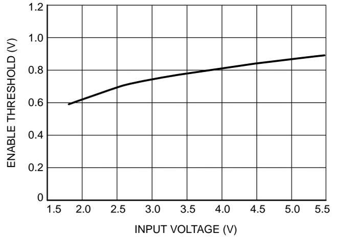
Figure 10. Falling Enable Threshold vs. Supply Voltage
