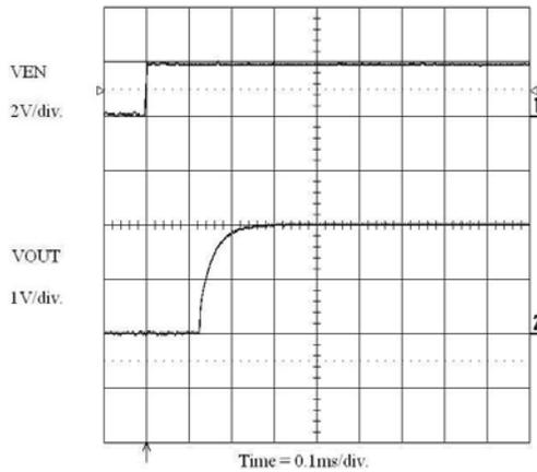
Figure 15. Enable Turn-On (1 mA Load)
