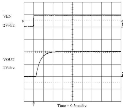
Figure 19. Enable Turn-On (1 mA Load)
