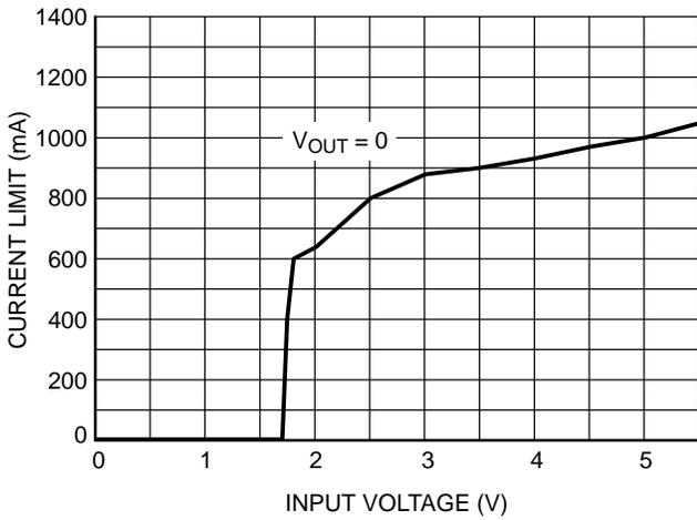
Figure 11. Current Limit on Output vs. Supply Voltage
