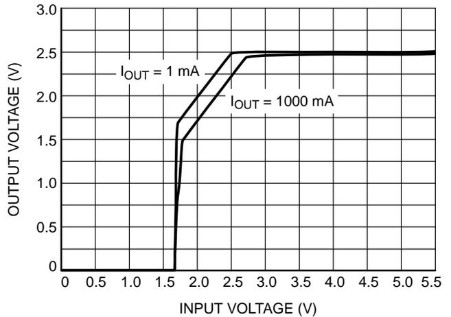
Figure 8. Dropout Characteristics
