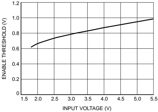
Figure 9. Rising Enable Threshold vs. Supply Voltage
