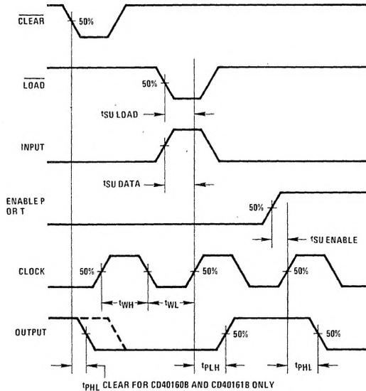
Note 1: All input pulses are from generators having the following characteristics:  $t_r = t_f = 20$  ns PRR  $\leq$  1 MHz duty cycle  $\leq$  50%,  $Z_{OUT} \approx 50\Omega$ .
