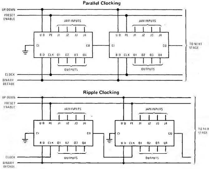
Carry out lines at the 2nd or later stages may have a negative-going spike due to differential internal delays. These spikes do not affect counter operation, but if the carry out is used to trigger external circuitry the carry out should be gated with the clock.
