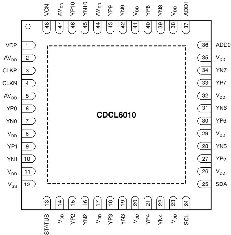
NOTE: Exposed thermal pad must be soldered to  $V_{SS}$ .
