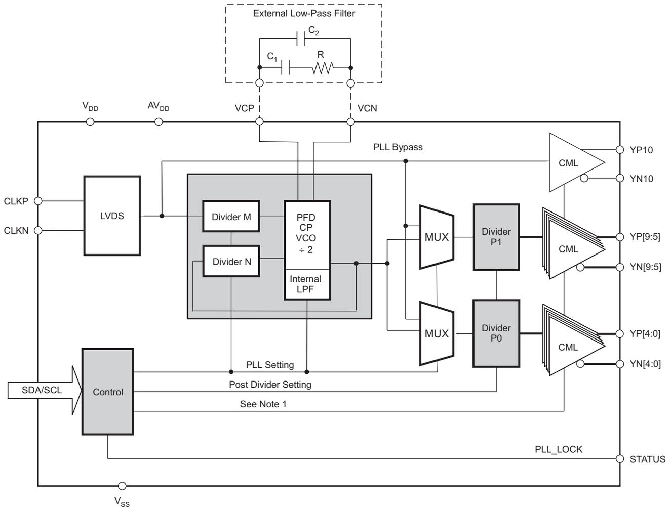
(1) Outputs can be disabled to floating. When outputs are left floating, internal 50Ω termination to V<sub>DD</sub> pulls both YN and YP to V<sub>DD</sub>.
