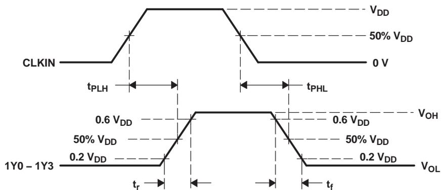
Figure 2. Voltage Waveforms Propagation Delay ( $t_{pd}$ ) Measurements
