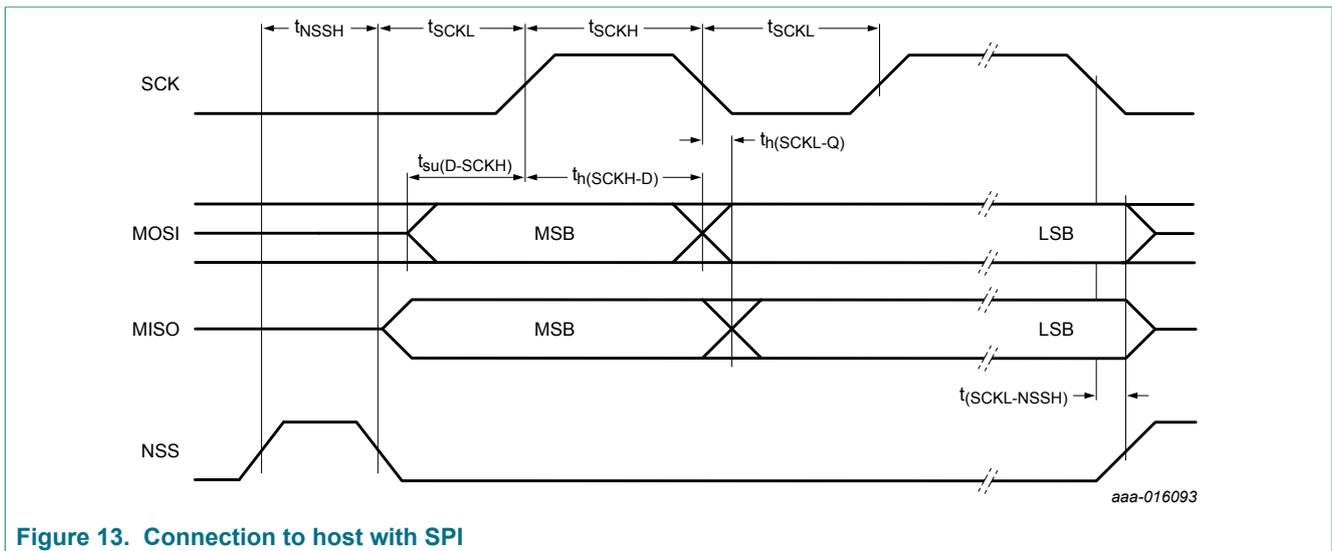
Figure 13. Connection to host with SPI
