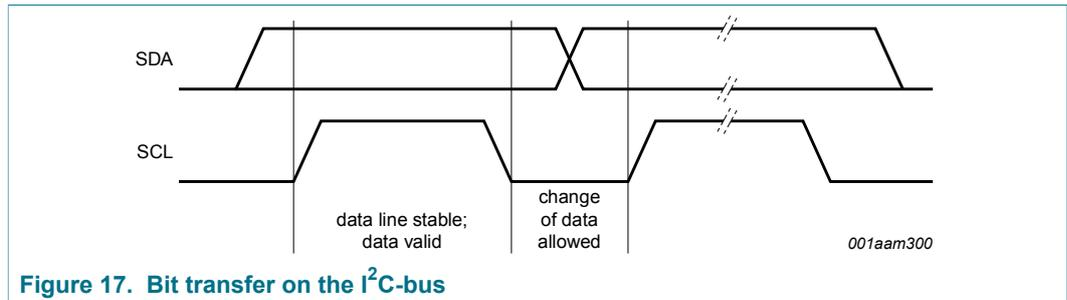
Figure 17. Bit transfer on the I<sup>2</sup>C-bus
