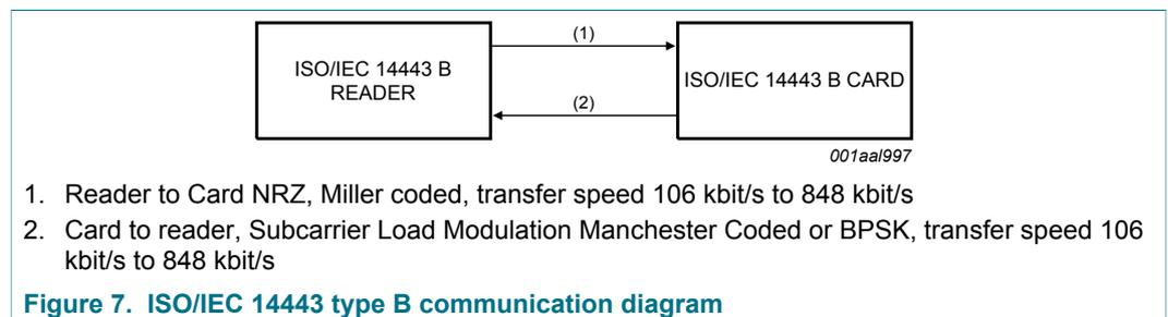
Figure 7. ISO/IEC 14443 type B communication diagram
