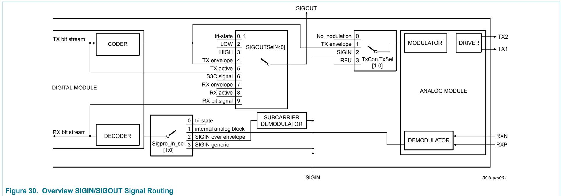
Figure 30. Overview SIGIN/SIGOUT Signal Routing
