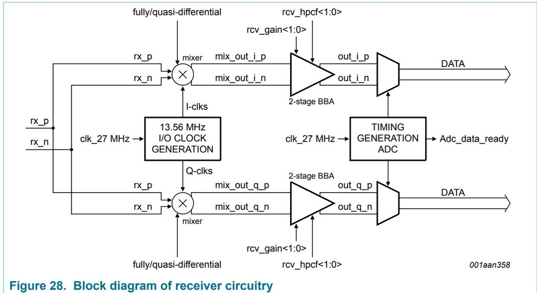
Figure 28. Block diagram of receiver circuitry
