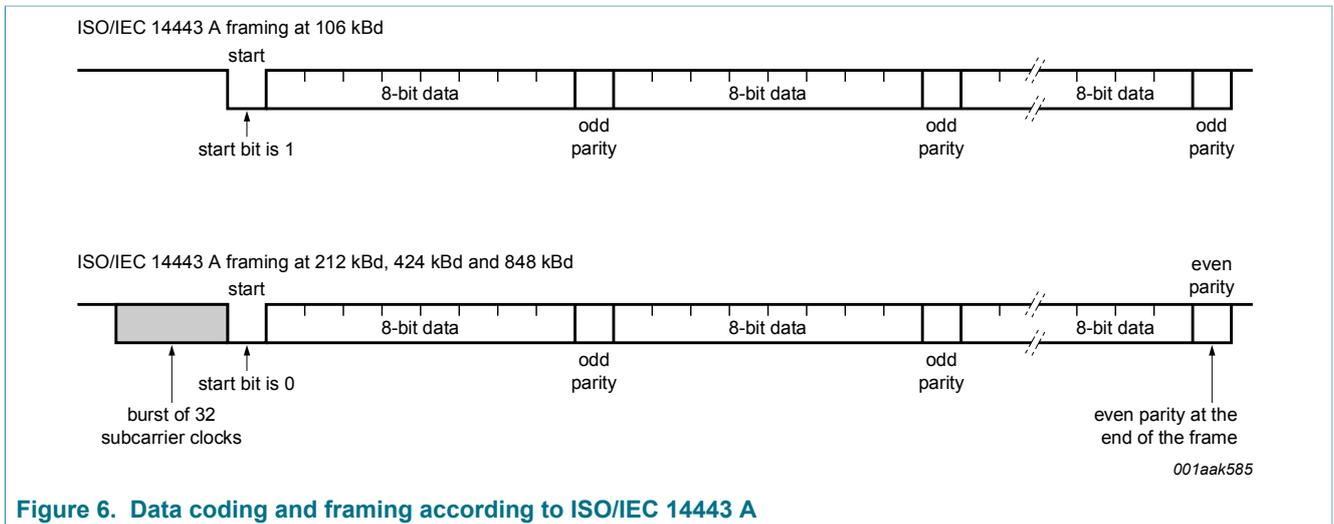
Figure 6. Data coding and framing according to ISO/IEC 14443 A
