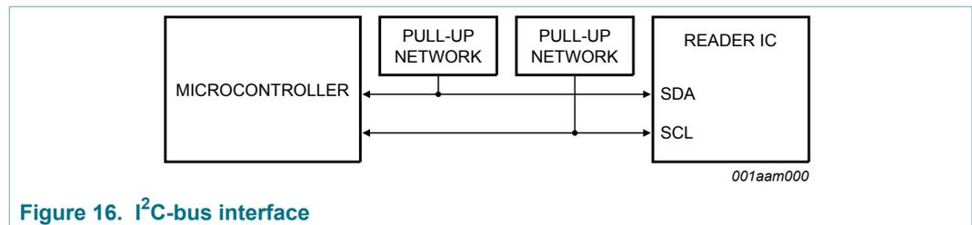
Figure 16. I<sup>2</sup>C-bus interface
