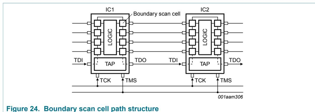
Figure 24. Boundary scan cell path structure
