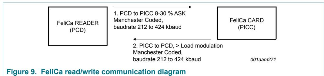
Figure 9. FeliCa read/write communication diagram
