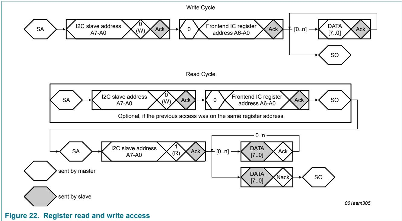
Figure 22. Register read and write access
