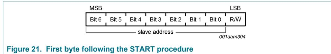
Figure 21. First byte following the START procedure
