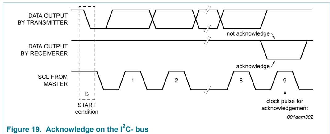
Figure 19. Acknowledge on the I<sup>2</sup>C-bus
