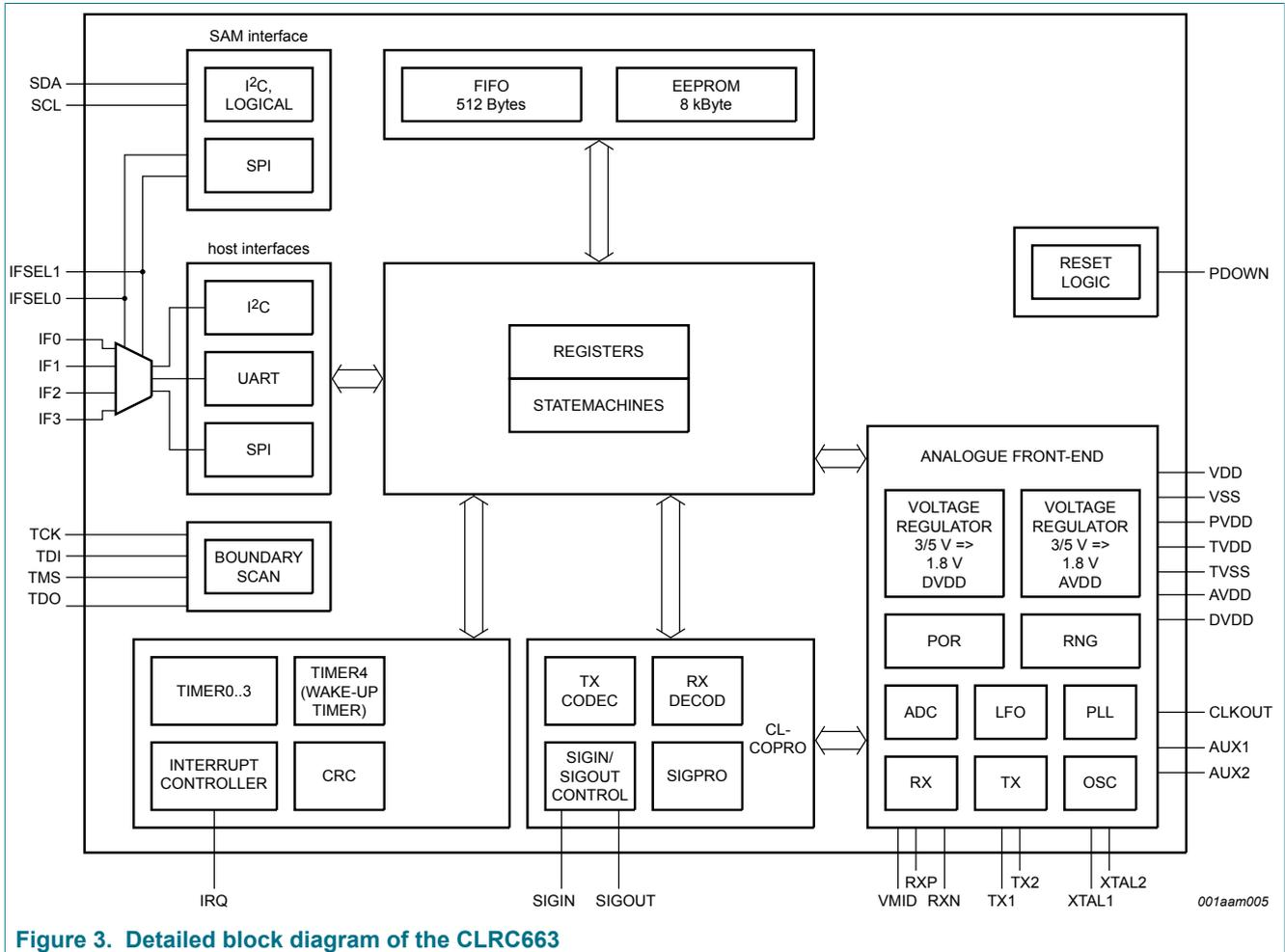
Figure 3. Detailed block diagram of the CLRC663
