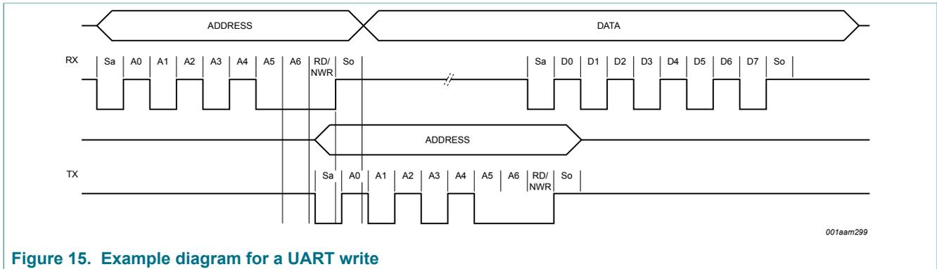
Figure 15. Example diagram for a UART write
