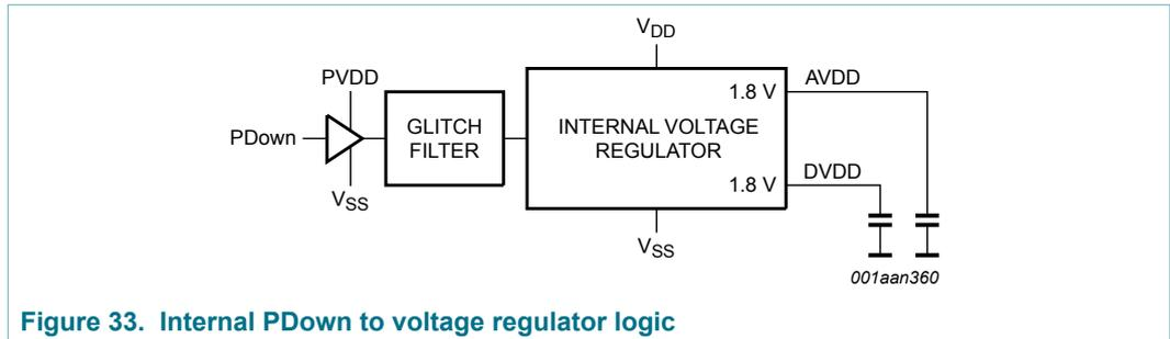
Figure 33. Internal PDown to voltage regulator logic
