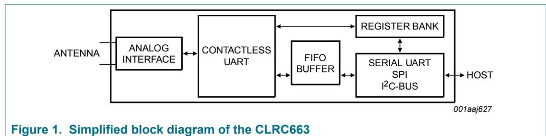
**Figure 1. Simplified block diagram of the CLRC663**
