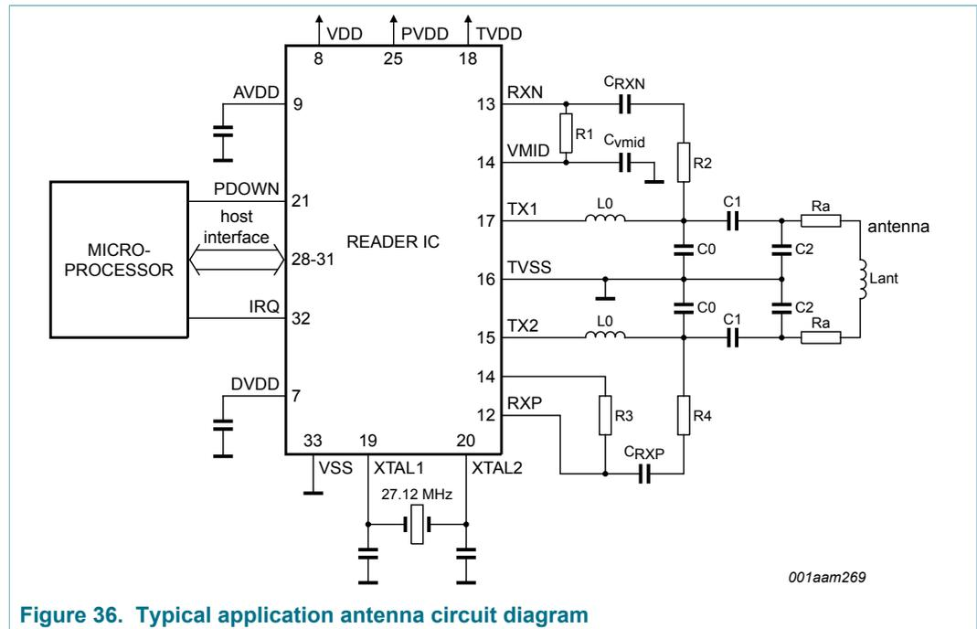
Figure 36. Typical application antenna circuit diagram
