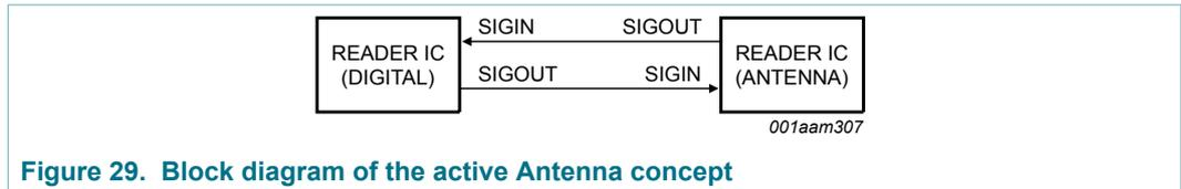
Figure 29. Block diagram of the active Antenna concept
