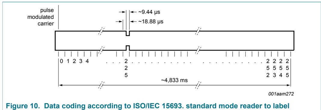
**Figure 10. Data coding according to ISO/IEC 15693. standard mode reader to label**
