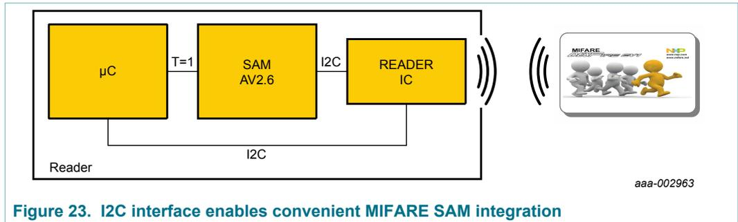
Figure 23. I2C interface enables convenient MIFARE SAM integration
