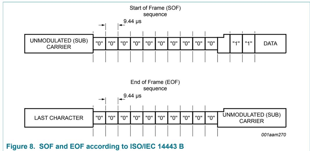
Figure 8. SOF and EOF according to ISO/IEC 14443 B
