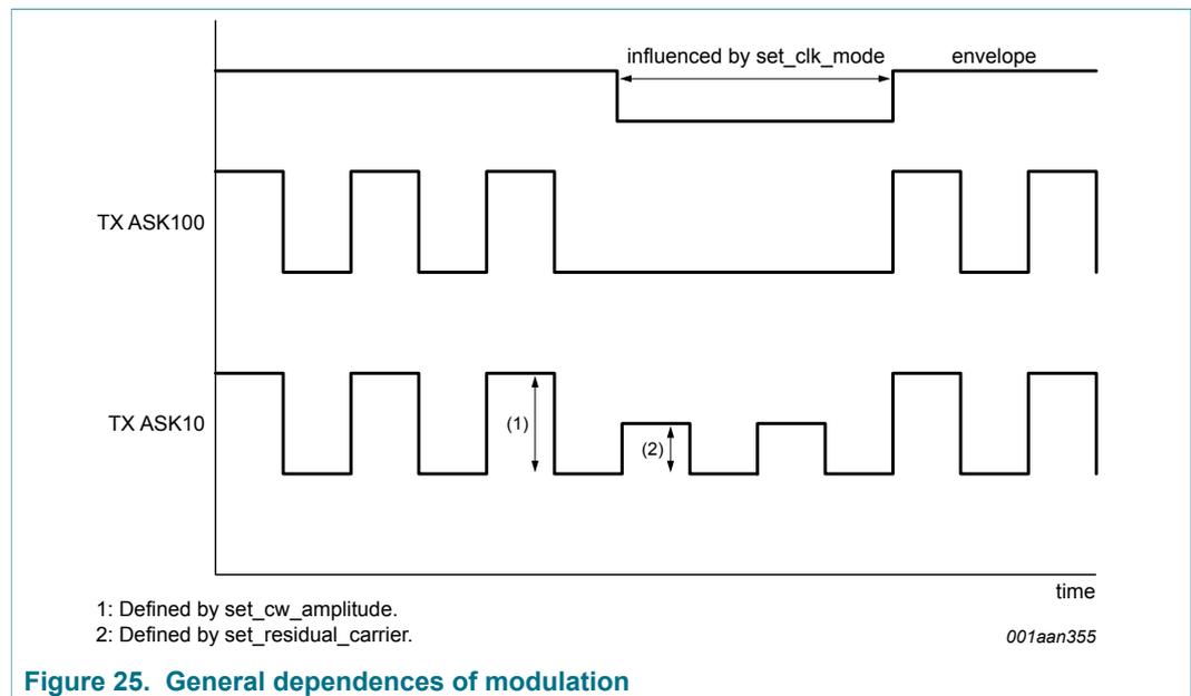
Note: When changing the continuous carrier amplitude, the residual carrier amplitude also changes, while the modulation index remains the same.
