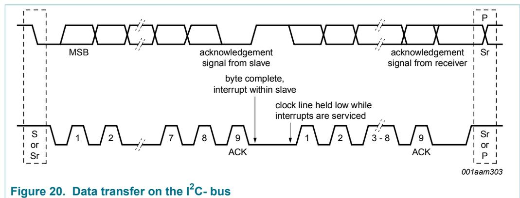
Figure 20. Data transfer on the I<sup>2</sup>C-bus
