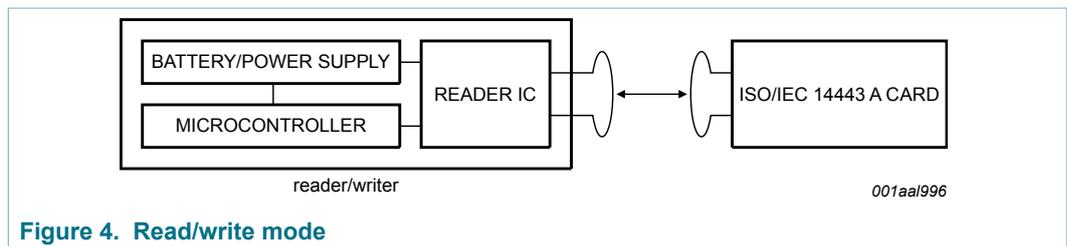
A typical system using the CLRC663 is using a microcontroller to implement the higher levels of the contactless communication protocol and a power supply (battery or external supply).
