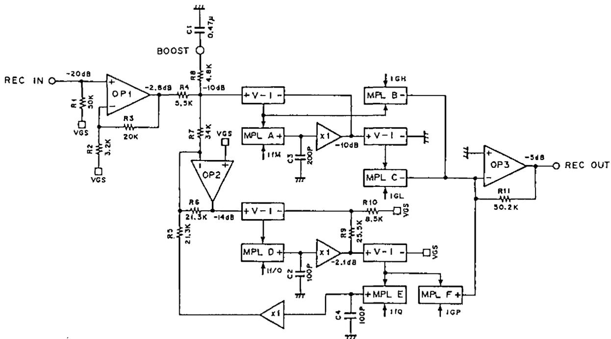
Fig. 1. CXA1578 functional circuit block diagram
