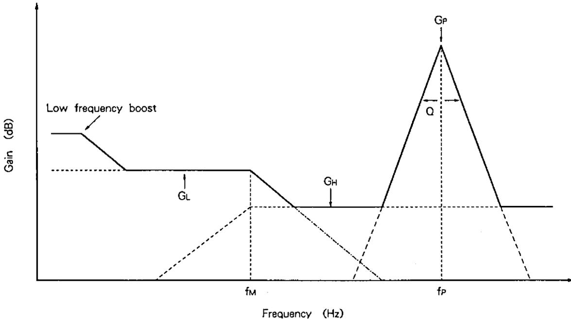
Fig. 2. Conceptual diagram of CXA1578 frequency characteristics
