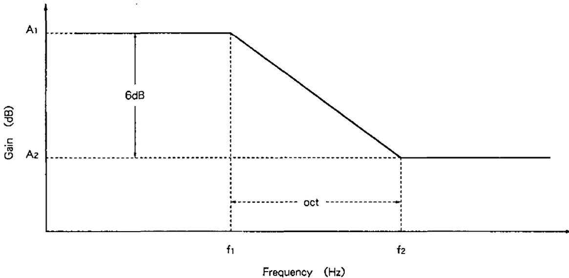
**Fig. 3. CXA1578 low frequency boost frequency characteristics**
