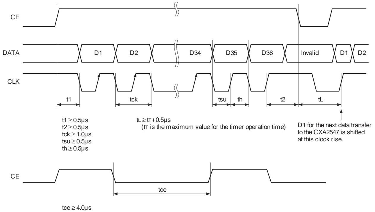
Timer Waiting Period Setting Chart ( $V_{CC}=7$  to  $12$  V, operating temperature= $-40$  °C to  $85$  °C)
