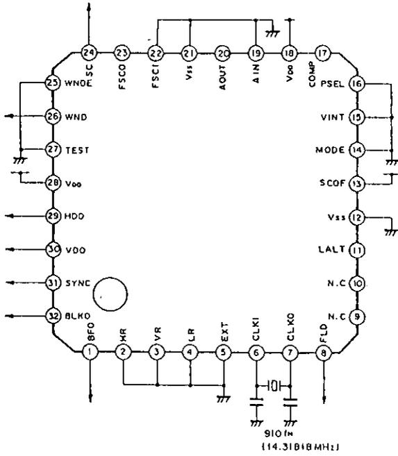
PAL (Filter configuration 2, Internal mode)
