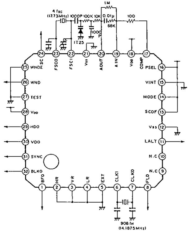
PAL (Filter configuration 1, Internal mode)
