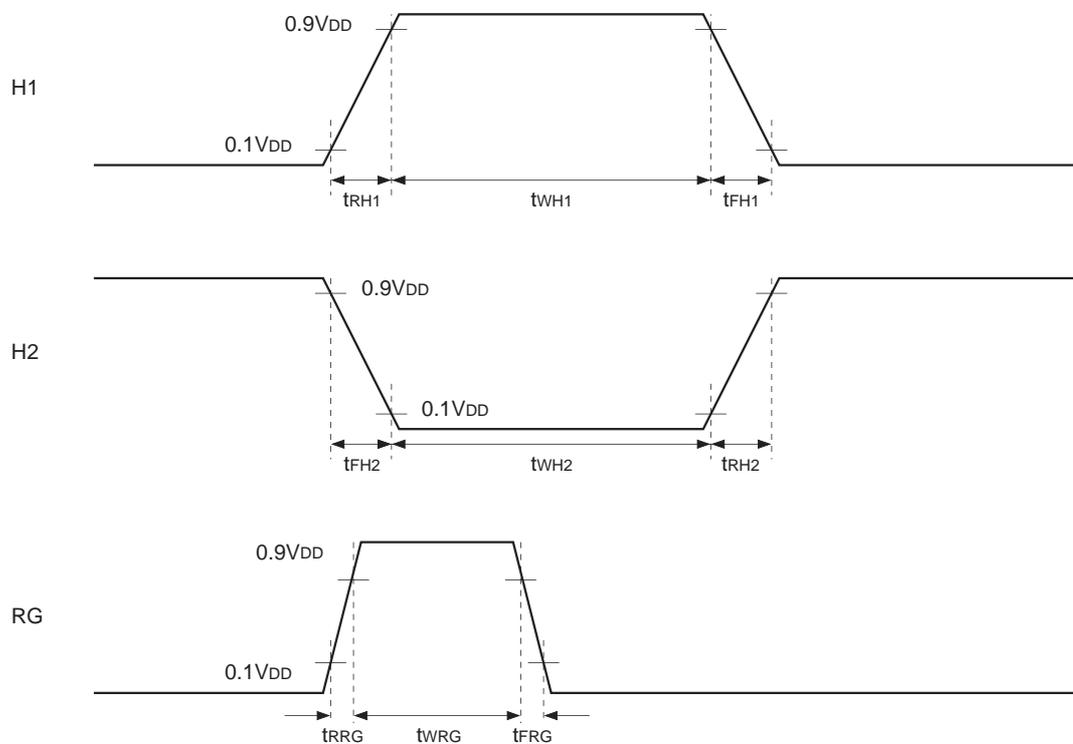
$V_{DD}=5.0$  V,  $T_{opr}=25$  °C, load capacitance of H1 and H2=100 pF, load capacitance of RG=10 pF
