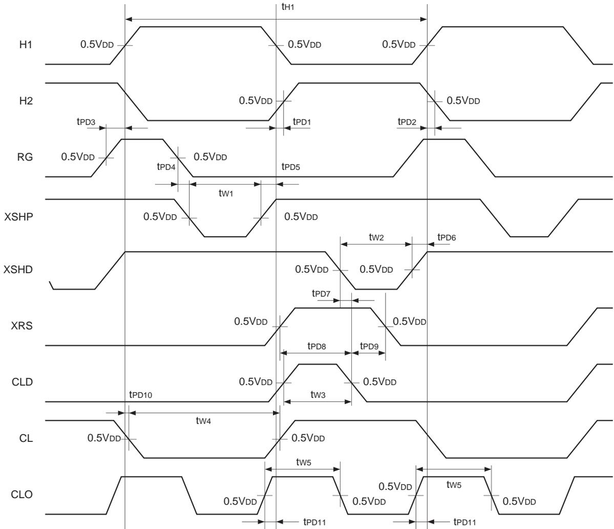
$V_{DD}=5.0\text{ V}$ ,  $T_{opr}=25\text{ }^{\circ}\text{C}$ , load capacitance of CL and CKO=30 pF, load capacitance of CLD, XSHP, XSHD, XRS and RG=10 pF
