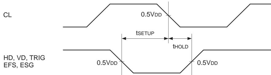
$V_{DD}=5.0\text{ V}$ ,  $T_{opr}=25\text{ }^{\circ}\text{C}$ , load capacitance of  $CL=30\text{ pF}$
