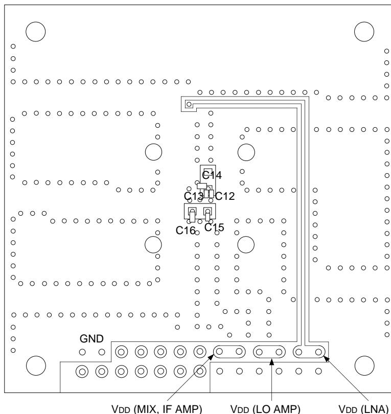
Glass fabric-base epoxy 4-layer board (2 × 0.3 mm thickness)
