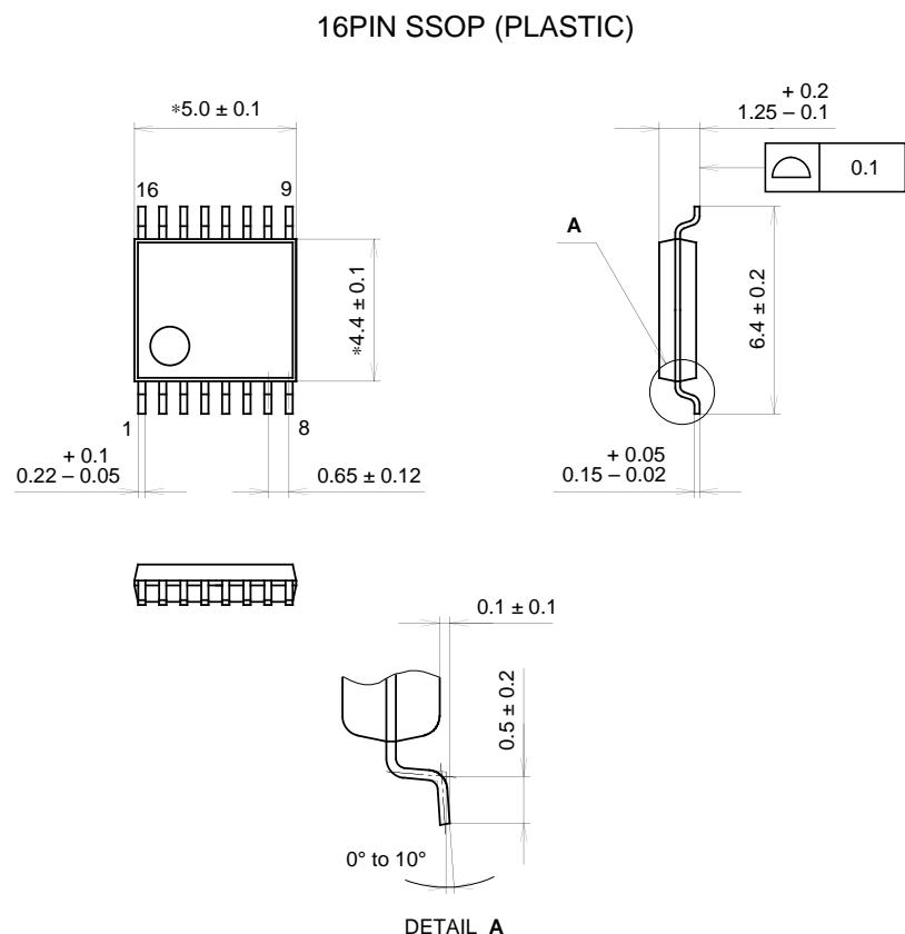
NOTE: Dimension "\*" does not include mold protrusion.
