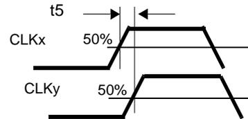
**Figure 10. Cycle to Cycle Jitter Definition (CCJ)**
