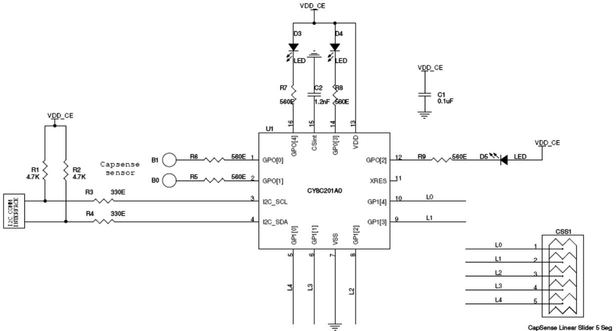
Figure 4. Circuit 2 – Compatibility with 1.8 V I<sup>2</sup>C Signaling [4, 5]
