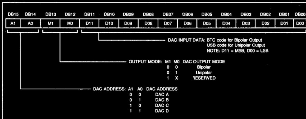
FIGURE 1. Serial Input Data Format.
