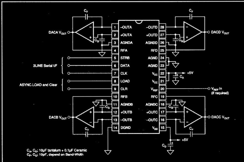
FIGURE 3. Typical I/V Amp Connection.
