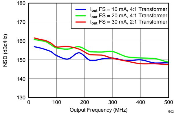
Figure 25. NSD vs Output Frequency Over  $I_{OUTFS}$
