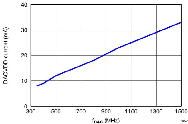
Figure 45. DACVDD Current vs  $f_{DAC}$  Over Interpolation
