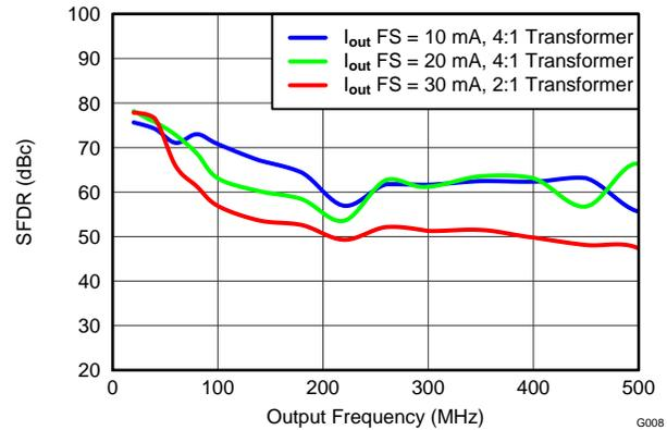
Figure 8. SFDR vs Output Frequency Over  $I_{OUT FS}$
