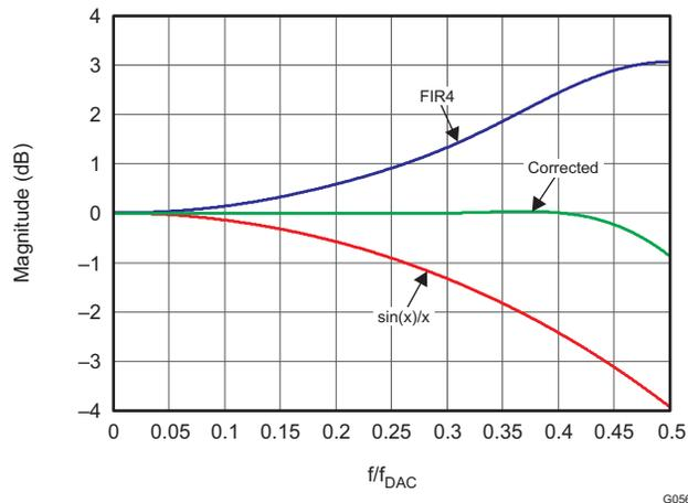
Figure 70. Magnitude Spectrum for Inverse Sinc Filter
