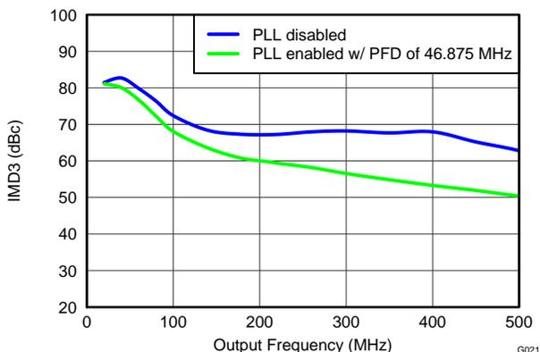
Figure 21. IMD3 vs Output Frequency Over Clocking Options
