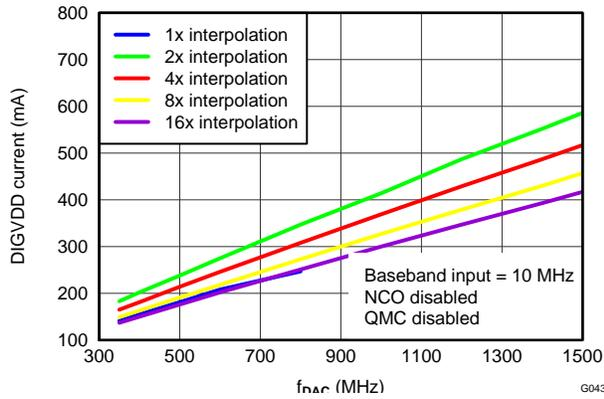
Figure 43. DIGVDD Current vs  $f_{DAC}$  Over Interpolation
