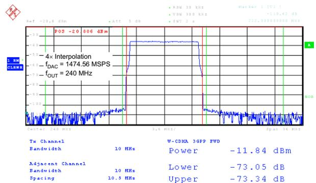
Figure 36. 10-MHz Single-Carrier LTE Test Mode3.1
