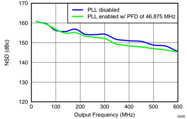
Figure 26. NSD vs Output Frequency Over Clocking Options
