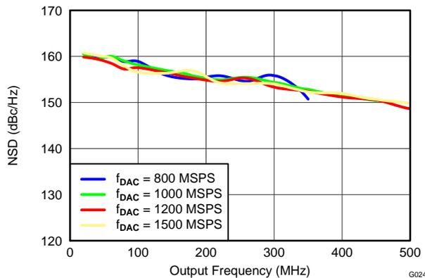
Figure 24. NSD vs Output Frequency Over  $f_{DAC}$
