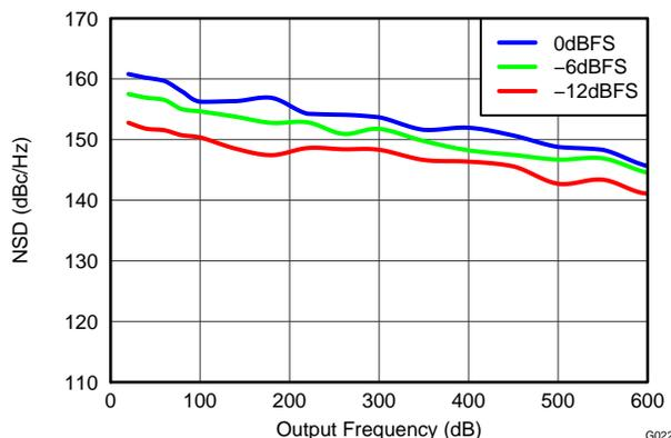
Figure 22. NSD vs Output Frequency Over Input Scale
