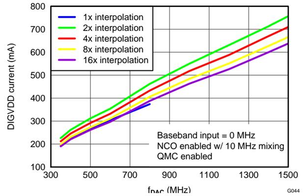
Figure 44. DIGVDD Current vs  $f_{DAC}$  Over Interpolation
