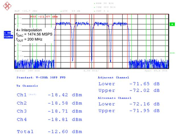
Figure 34. Four-Carrier WCDMA Test Mode1
