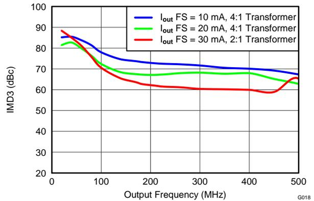
Figure 18. IMD3 vs Output Frequency Over  $I_{OUTFS}$
