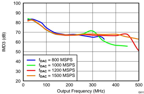
Figure 17. IMD3 vs Output Frequency Over  $f_{DAC}$
