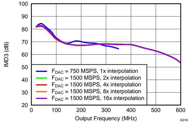
Figure 16. IMD3 vs Output Frequency Over Interpolation
