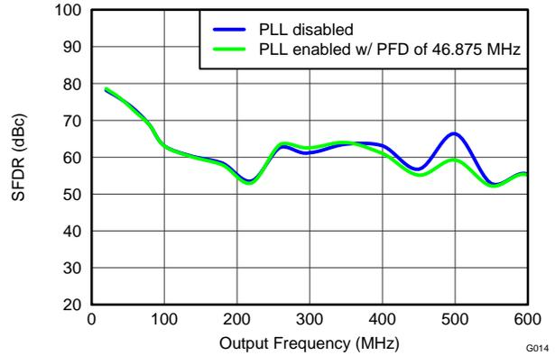
Figure 14. SFDR vs Output Frequency Over Cloning Options
