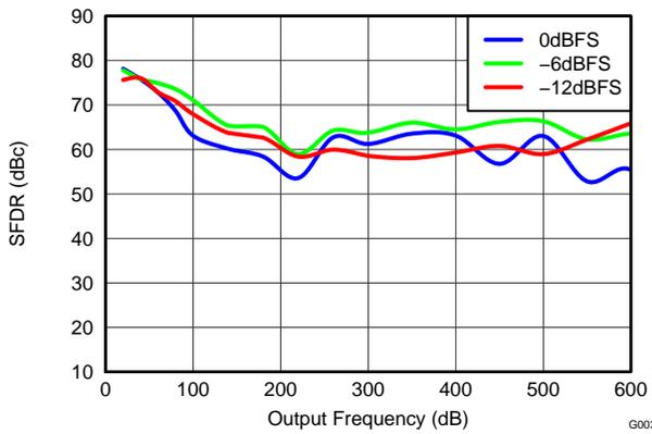
Figure 3. SFDR vs Output Frequency Over Input Scale
