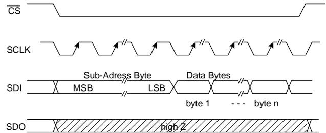
**Fig. 2–4:** SPI Control Port - Write Access
