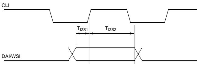
Fig. 4-15: I<sup>2</sup>S timing diagram
