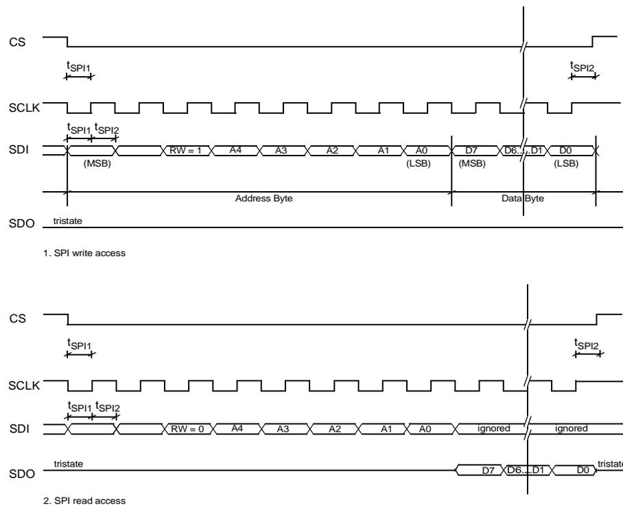
Fig. 4-16: SPI write and read access
