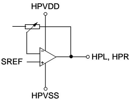
Fig. 4-8: Output Pins: HPL, HPR
