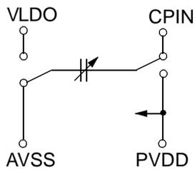
Fig. 4-4: Supply Pins: CPIN, PVDD
