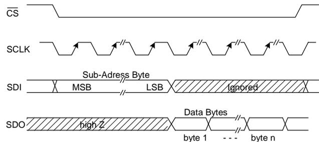
**Fig. 2–5:** SPI Control Port - Read Access
