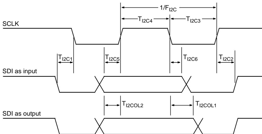
Fig. 4-14: I<sup>2</sup>C bus timing diagram
