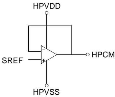
Fig. 4-7: Output Pin: HPCM
