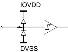
Fig. 4-9: Input Pins: Mode,  $\overline{CS}$ , DAI, WSI, CLI,  $\overline{RES}$
