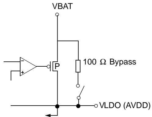
Fig. 4-5: Supply Pins: VLDO, VBAT
