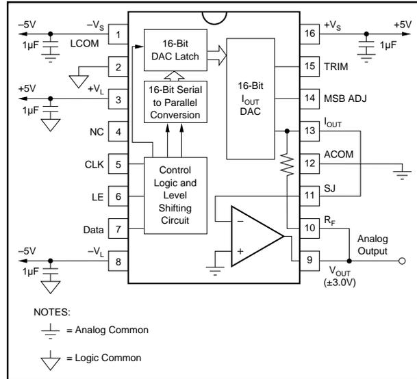
FIGURE 2. Connection Diagram.
