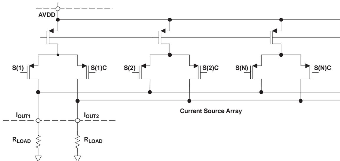
Figure 18. Analog Outputs
