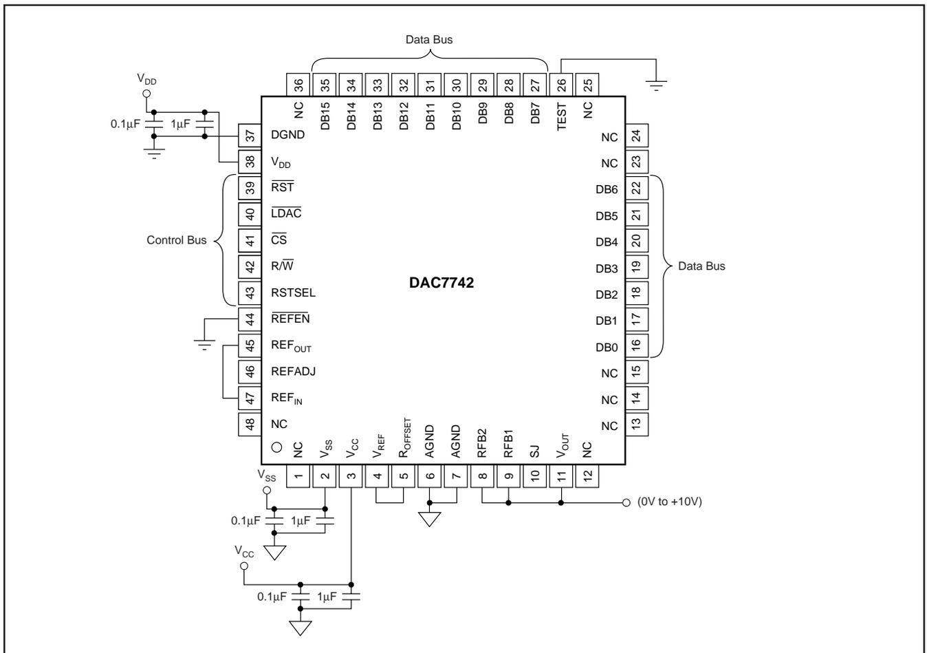
FIGURE 2. Basic Operation:  $V_{\text{OUT}} = 0\text{V}$  to +10V.
