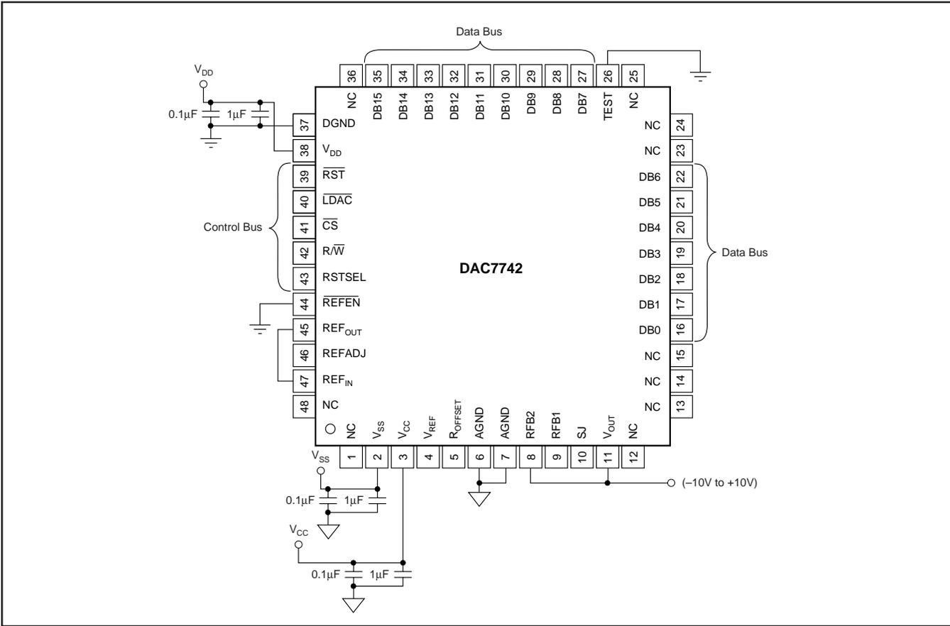
FIGURE 4. Basic Operation: V<sub>OUT</sub> = -10V to +10V.
