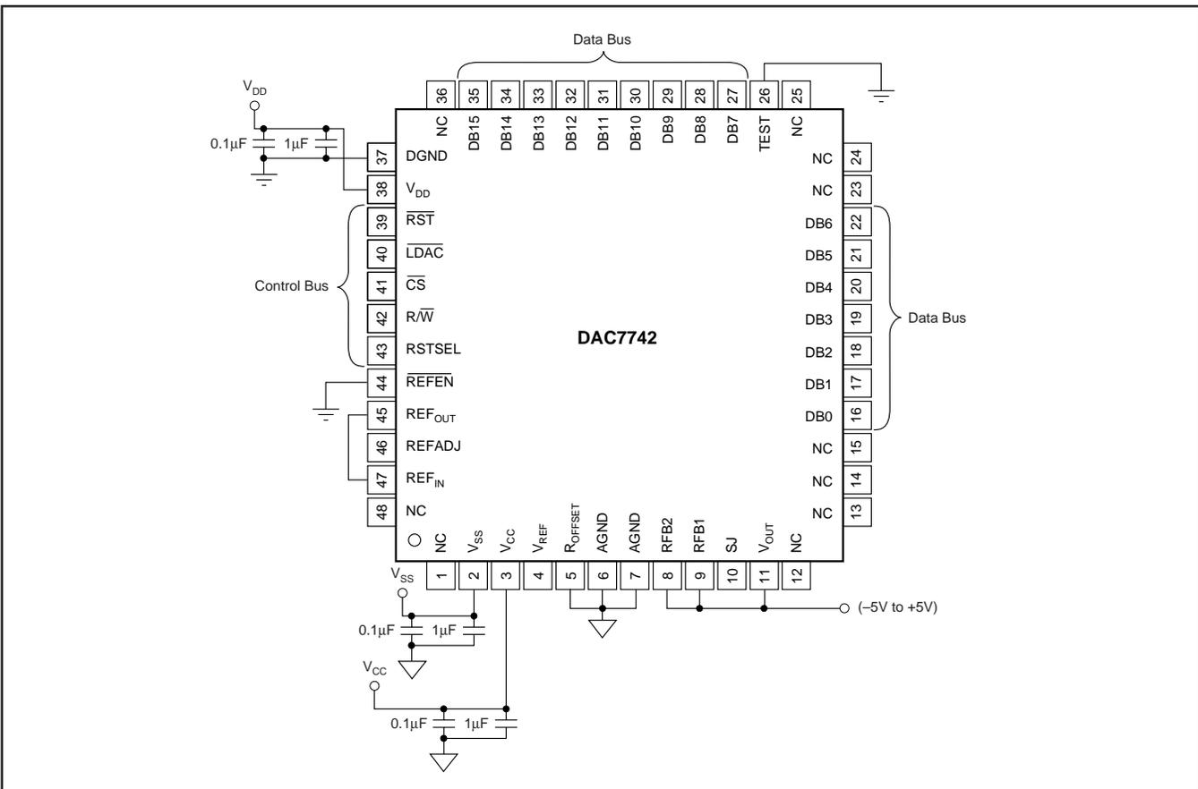
FIGURE 3. Basic Operation: V<sub>OUT</sub> = -5V to +5V.
