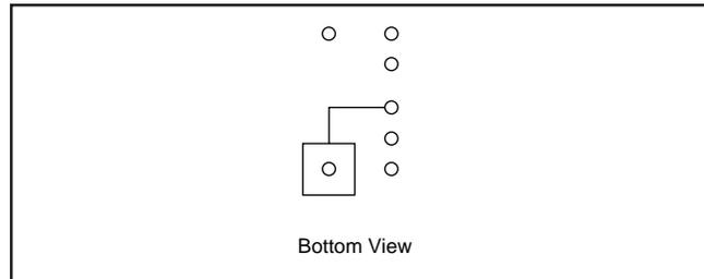
FIGURE 2. SYNC<sub>OUT</sub> Guard Ring.
