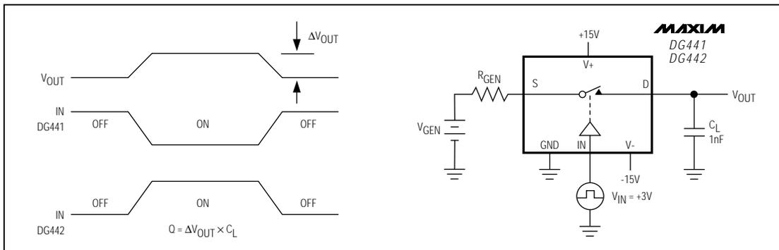
Figure 3. Charge Injection
