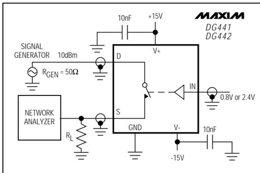
Figure 4. Off-Isolation Rejection Ratio
