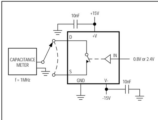
Figure 6. Source/Drain-On/-Off Capacitance
