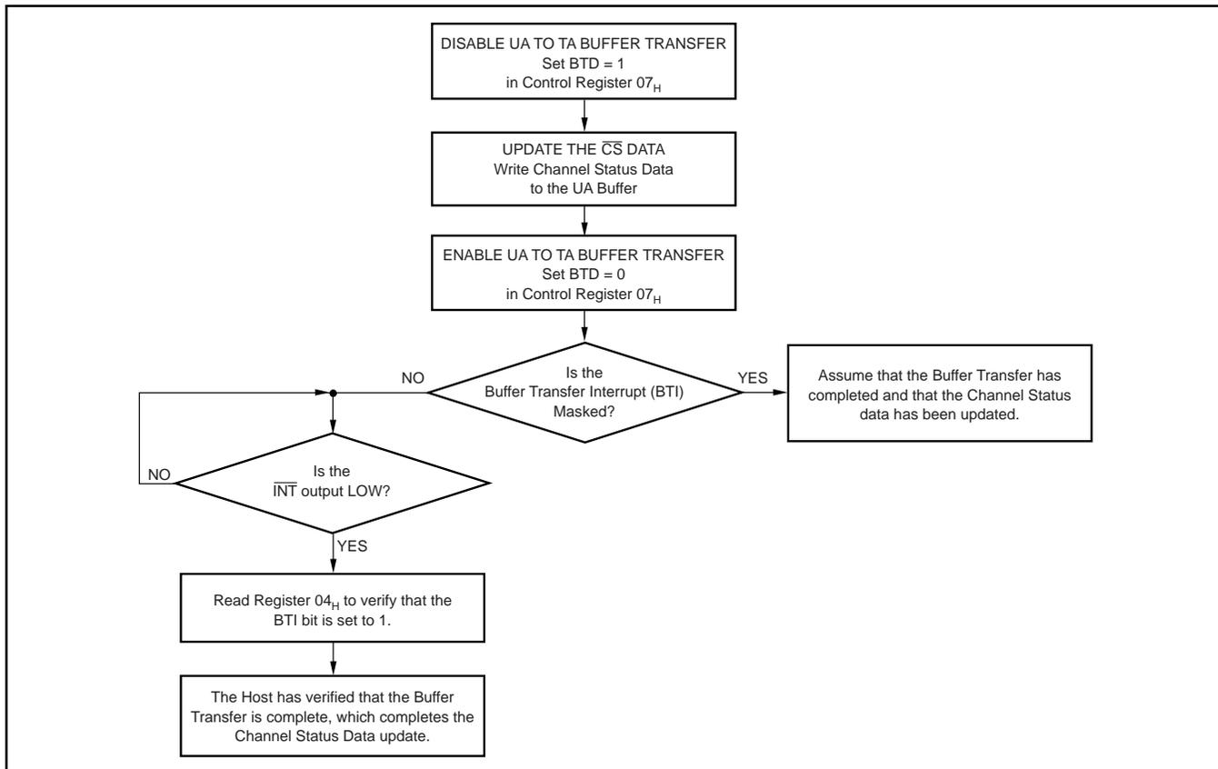
FIGURE 9. Flowchart for Updating the Channel Status Buffer.
