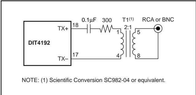
FIGURE 13. Recommended Transmitter Output Circuit for Unbalanced, 75Ω Coaxial Cable Transmission.
