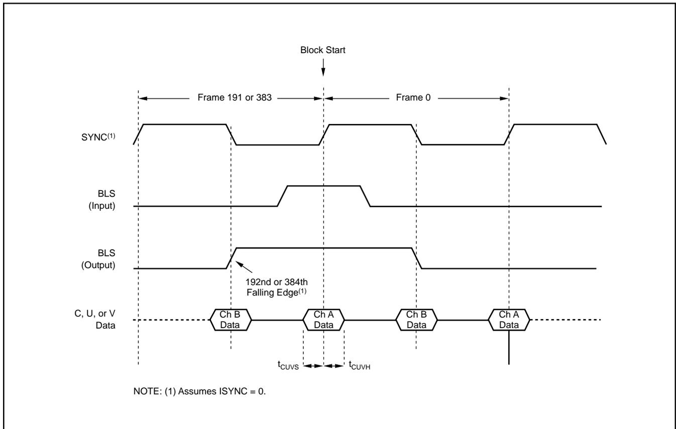
FIGURE 5. C, U, and V Data Timing.
