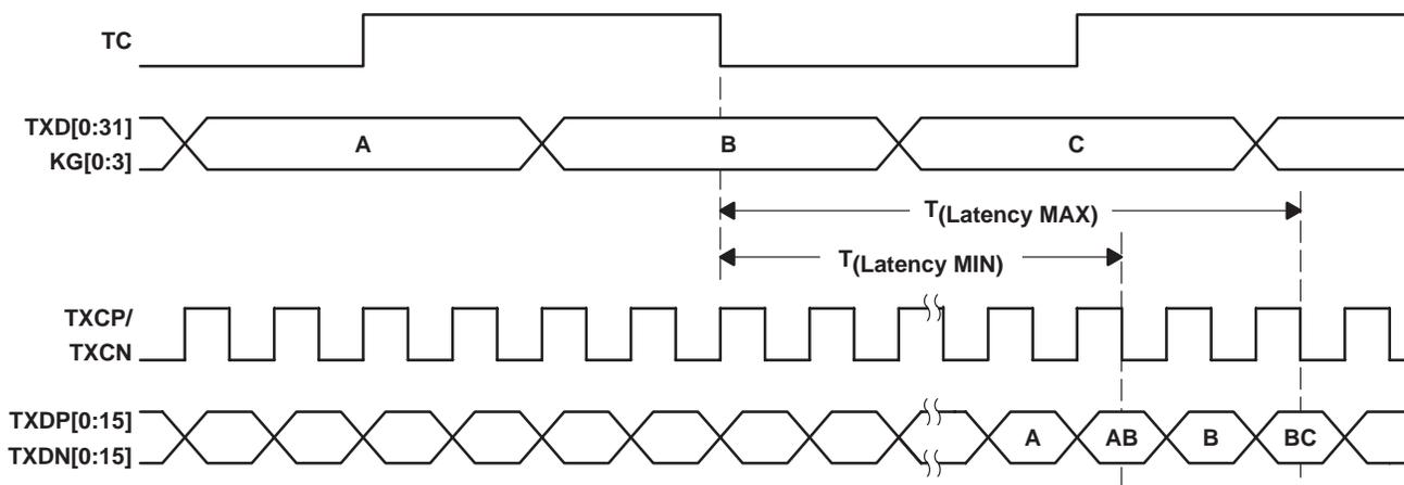
Figure 6. Transmitter Latency
