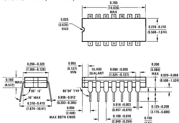
**14-Lead Ceramic Dual-In-Line Package (J)**
