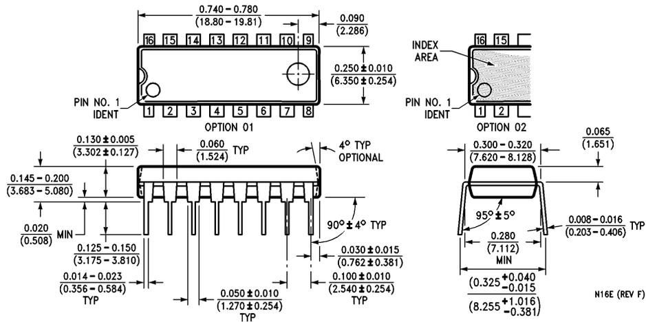
**16-Lead Molded Dual-In-Line Package (N)**
