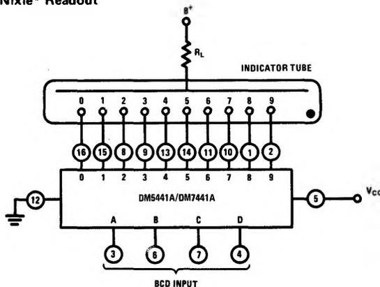
NOTE: Values for B+ and  $R_L$  are as specified by the tube manufacturer.
