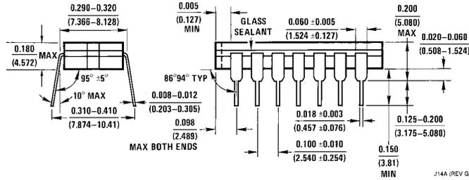
**14-Lead Ceramic Dual-In-Line Package (J)**
