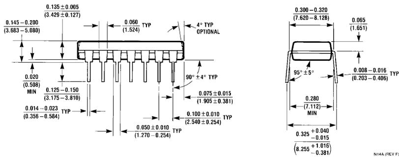
**14-Lead Molded Dual-In-Line Package (N)**
