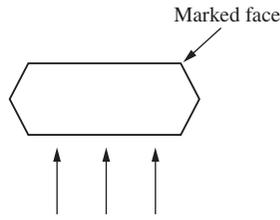
Applying direction of magnetic flux
