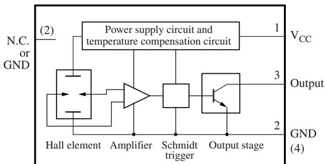
Note) The number in ( ) shows the pin number for the DN6849S.
