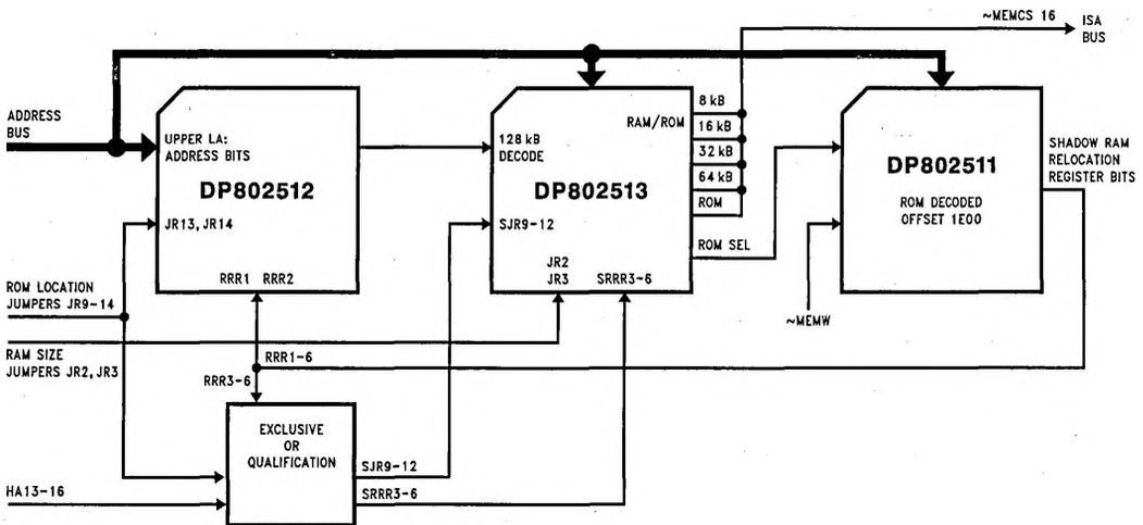
FIGURE 2. MEMCS\_16 Logic
