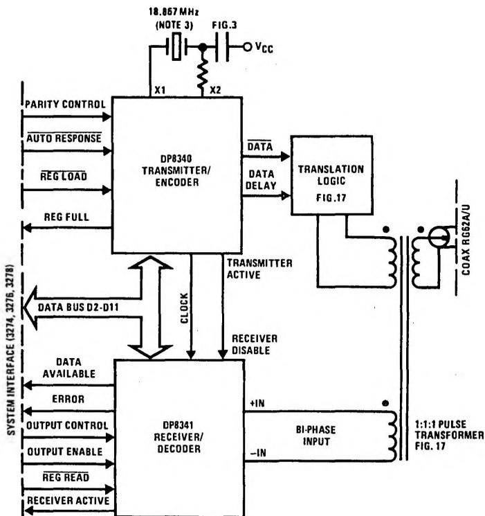
FIGURE 16. Typical Applications for IBM 3270 Interface
