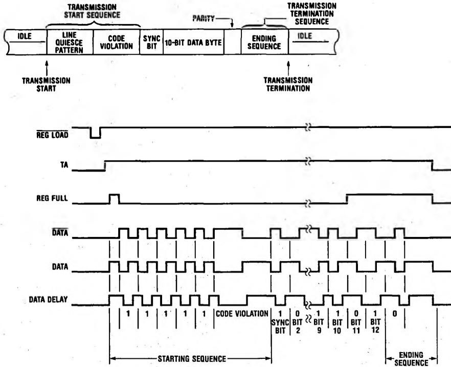
FIGURE 4. Overall Timing Waveforms for Single Byte
