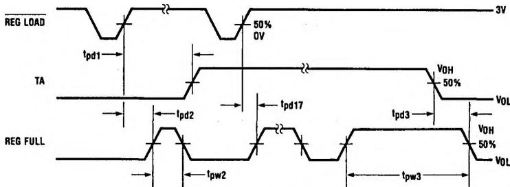
FIGURE 14. Timing Waveforms for Two Byte Transfer
