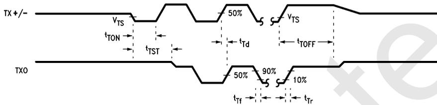
FIGURE 6. Transmitter Timing
