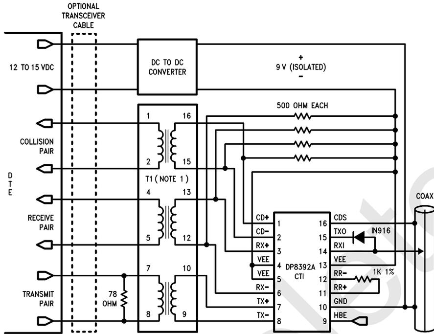
**Note 1:** T1 is a 1:1 pulse transformer,  $L = 100 \mu\text{H}$
