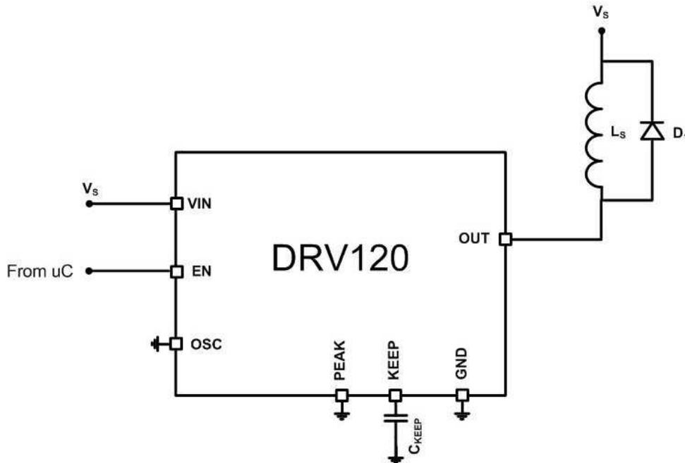
Figure 1. Default Configuration With 8-Pin TSSOP Option
