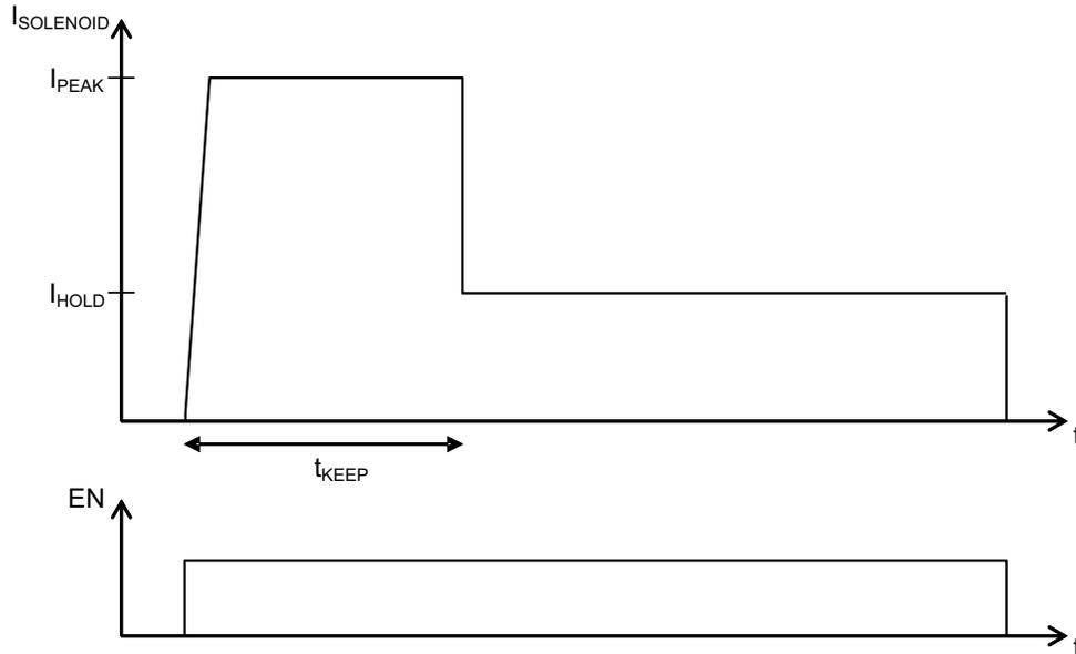
**Figure 3. Typical Current Waveform Through the Solenoid**
