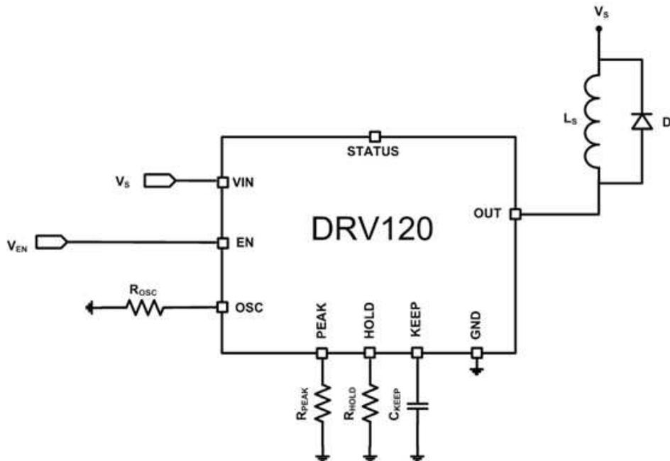
Figure 2. External Parameter Setting for 14-Pin TSSOP Option
