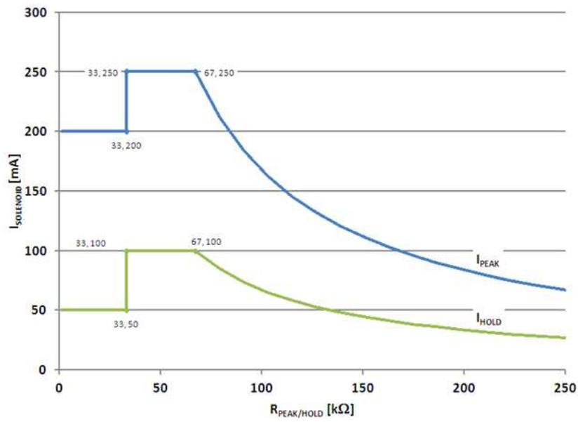
Figure 4. PEAK and HOLD Mode Current Settings
