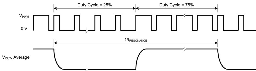
Figure 14. LRA Example for 1/2 Full-Scale Drive
