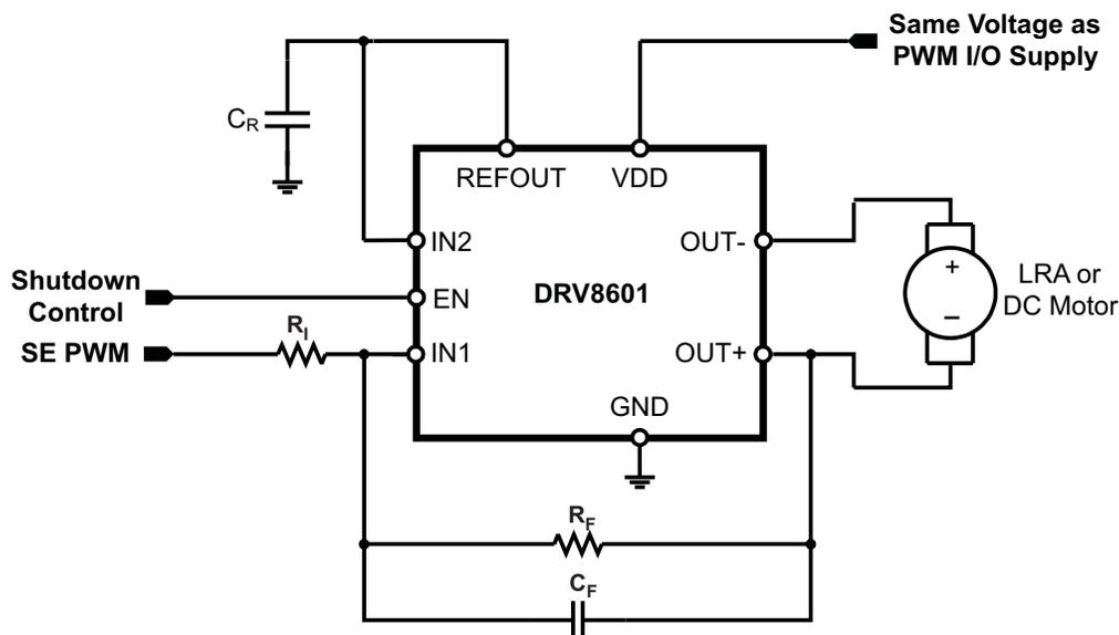
Figure 15. Pseudo-Differential Feedback with Internal Reference
