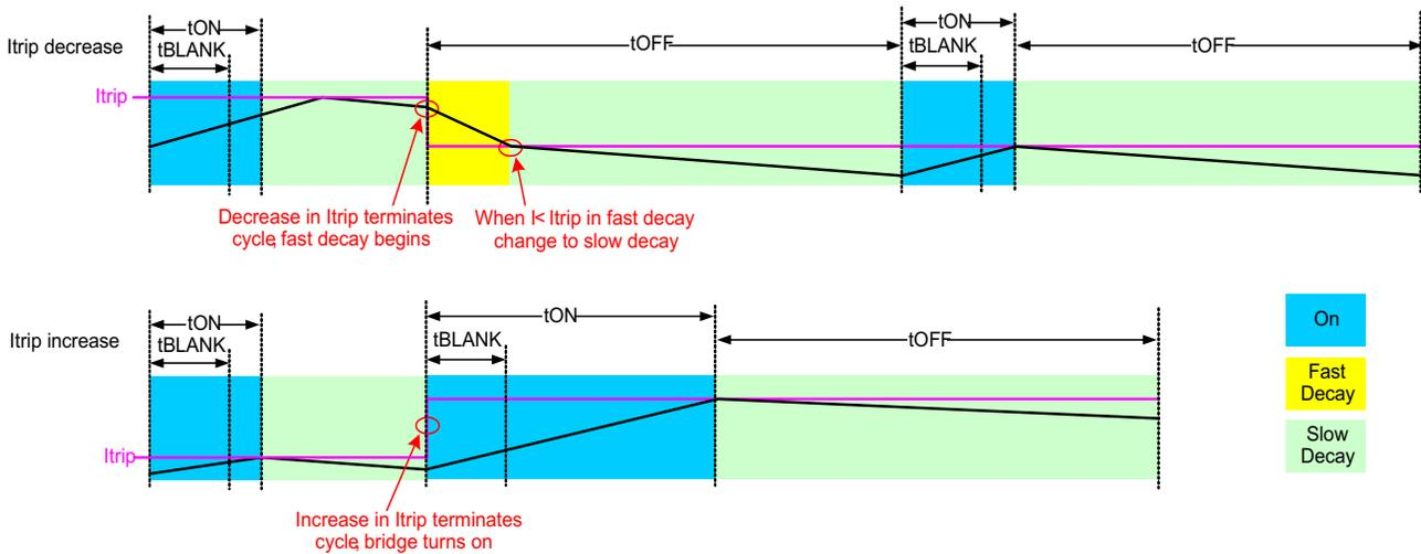
Figure 11. Itrip Level Changing During a PWM Cycle
