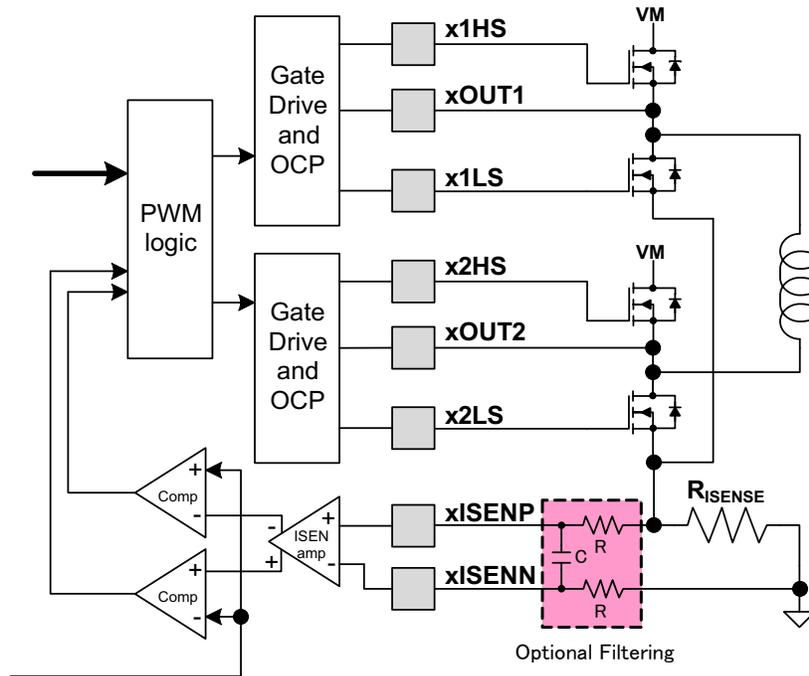
Figure 12. Optional Filtering Between  $R_{ISENSE}$  and xINSENx
