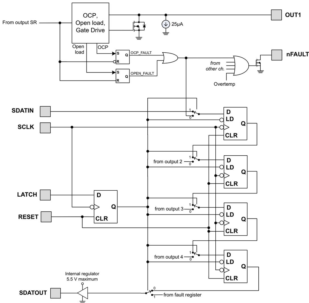
Figure 7. Fault Output
