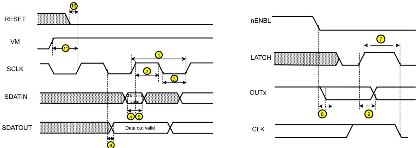
More than 400 ns of delay should exist between the final SCLK rising edge and the LATCH rising edge. This ensures that the last data bit is shifted into the device properly.
