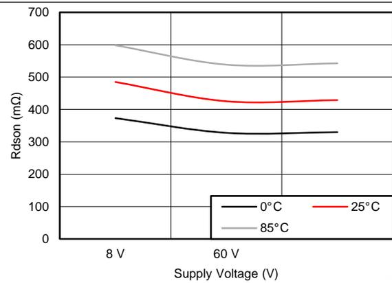
Figure 5.  $R_{DS(ON)}$  vs Supply Voltage
