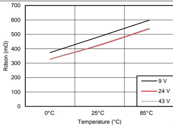
Figure 4.  $R_{DS(ON)}$  vs Temperature
