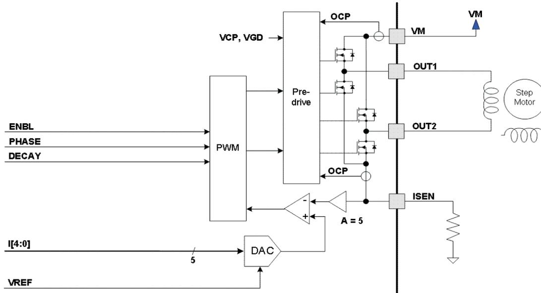
Figure 1. Motor Control Circuitry
