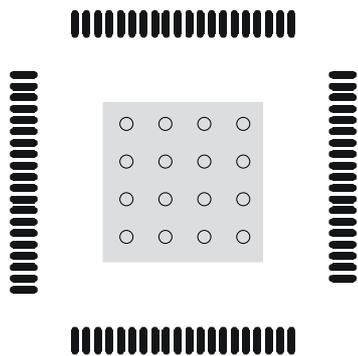
**Fig. 2–6:** Thermal via array
