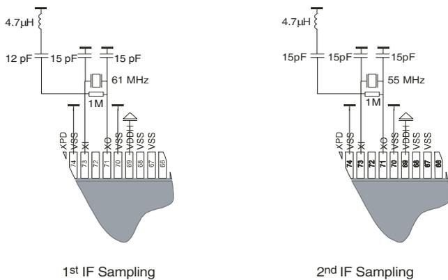
**Fig. 2-4:** Clocking circuitry for 1<sup>st</sup> IF or baseband sampling
