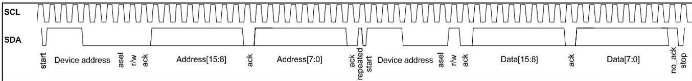
Fig. 2–9: I2C\_Read timing (NrOfBytes = 2)
