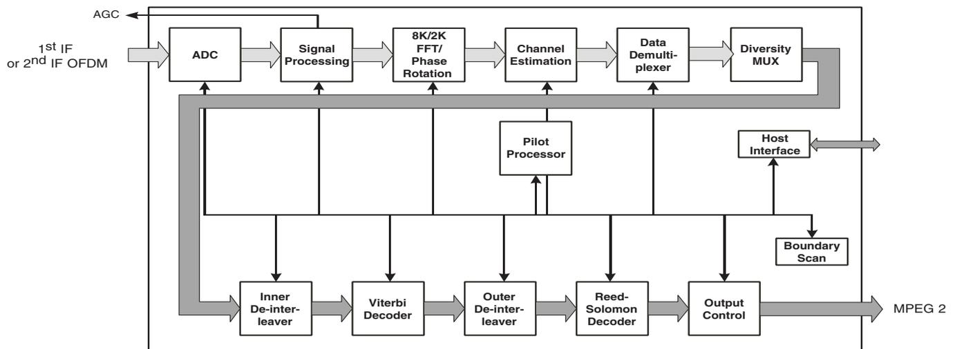
**Fig. 1-1:** Block diagram of the DRX 8872C
