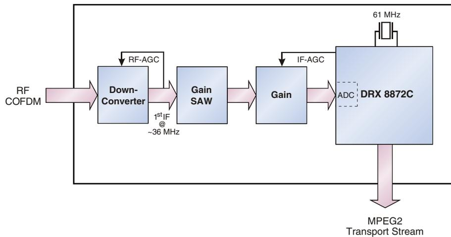
**Fig. 1–2:** Front-end block diagram for the DRX 8872C
