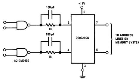
Figure 7. DC Coupled RAM Memory Address or Precharge Driver (Positive Supply Only)
