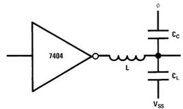
Figure 10. Clock Coupling
