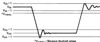
**Figure 8. Clock Waveform**
