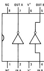
Figure 1. (Top View) Dual-In-Line Package
