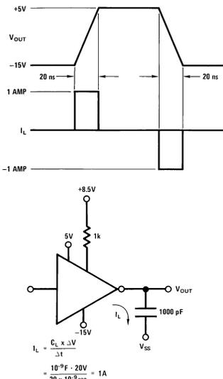
**Figure 9. Clock Waveforms (Voltage and Current)**
