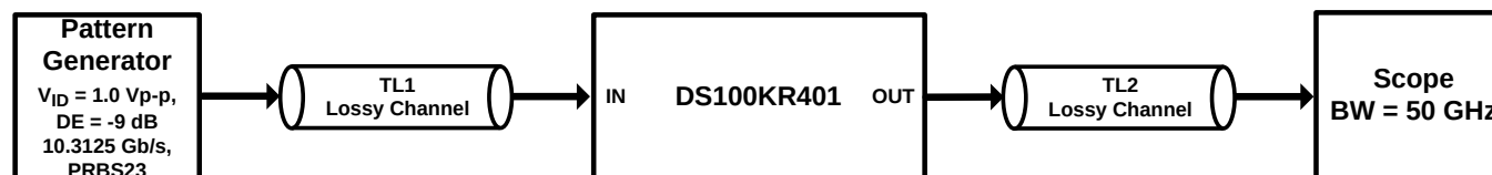
Figure 13. Test Setup Connections Diagram
