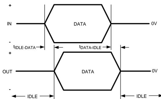
Figure 4. Transmit IDLE-DATA and DATA-IDLE Response Time
