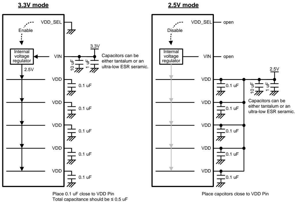
Figure 6. 3.3V or 2.5V Supply Connection Diagram
