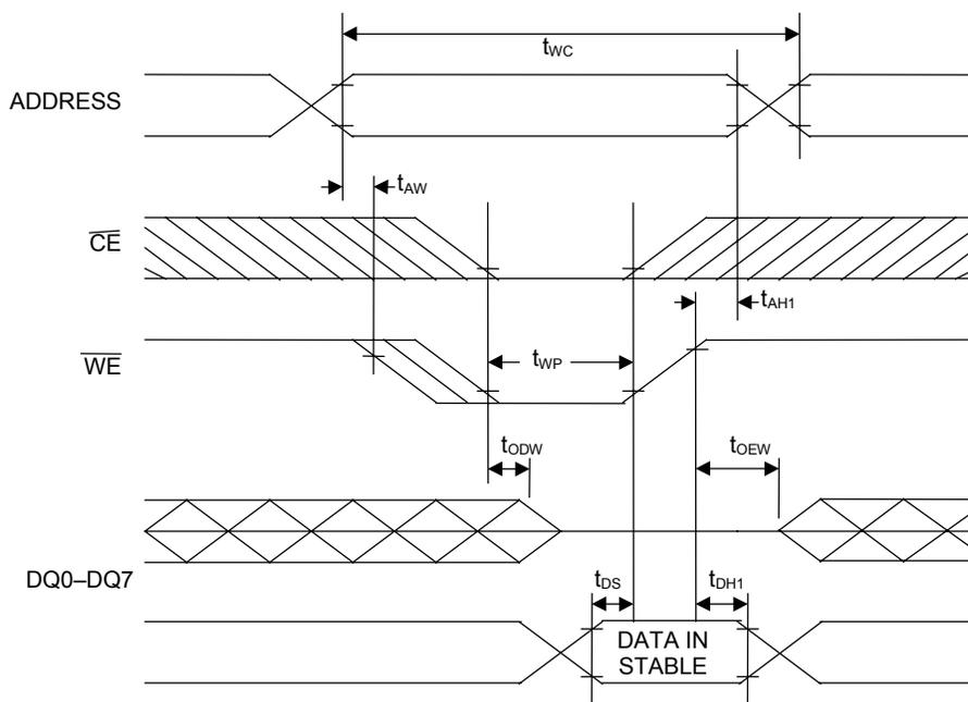
**Figure 6. MEMORY WRITE CYCLE TIMING, CHIP-ENABLE CONTROLLED**
